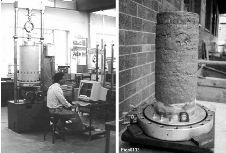
Figure 4 – Triaxial test equipment and a rockfill sample
