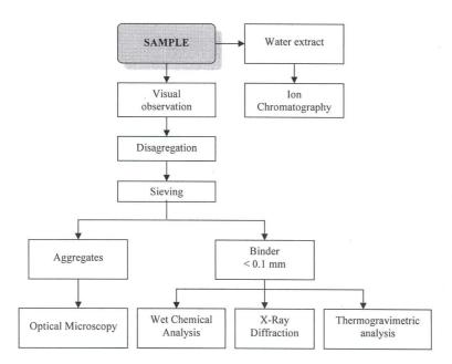
Figure 6. Flowchart of Roman mortar characterization
