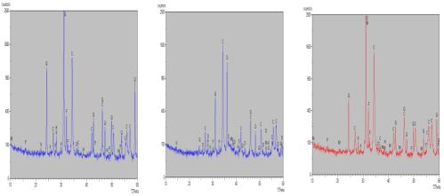
Figure 7. X-ray diffraction patterns of samples 2, 5 and 20 (from left to right)
