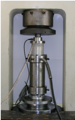
Figure 7: Triaxial test assembly of the core with the cell
