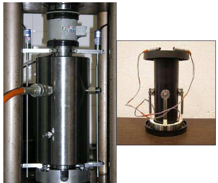
Figure 2. Triaxial cell and internal sleeve with diametral displacements transducers.
