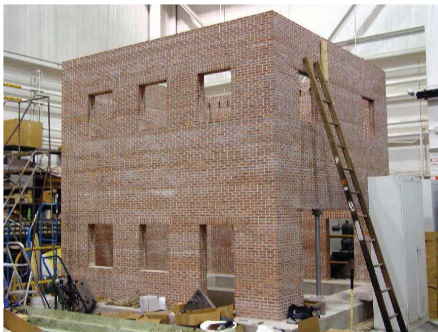
Figura 2.62 – Vista do modelo ensaiado no Construction Engineering Research Laboratory (CERL) do U.S. Army Engineer Research and Development Center (ERDC), U.S. Army Corps of Engineers (USA CE) [Sweeney et al. , 2004]
