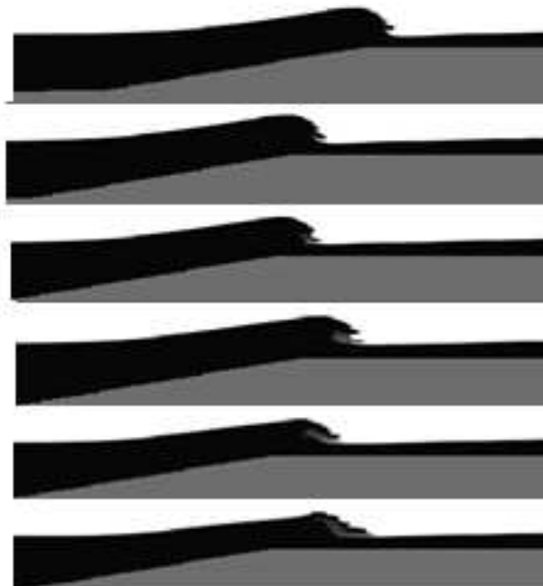
Figure 4.21 - Wave shape on the reef with a slope of 1:6 (after 62 s, wave 3).
