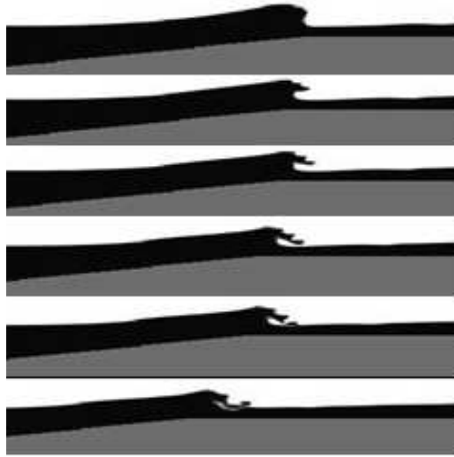
Figure 4.22 - Wave shape on the reef with a slope of 1:10 (after 62 s, wave 3).
