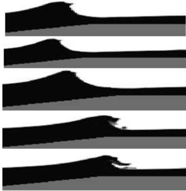
Figure 4.15 - Wave shape on the reef with a height of 1.90 m (after 62 s, wave 3).
