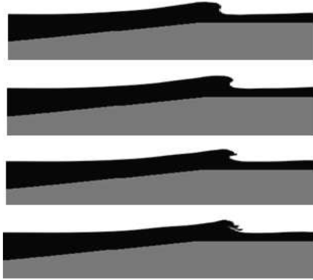
Figure 4.31 - Wave shape on the reef with a submergence of 2.0 m (after 63 s, wave 3).
