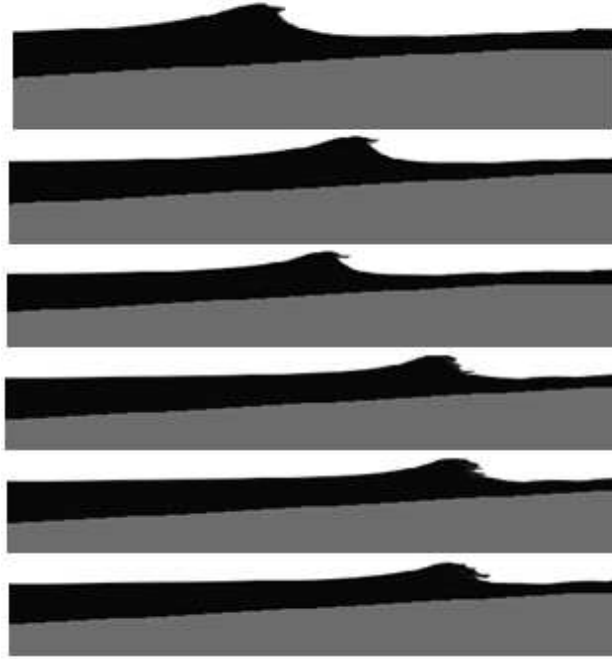
Figure 4.24 - Wave shape on the reef with a slope of 1:18 (after 62 s, wave 3).
