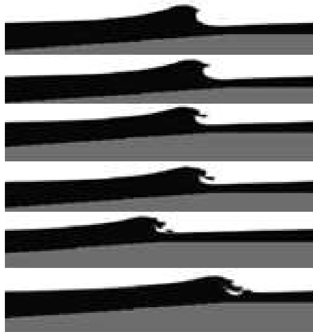
Figure 4.23 - Wave shape on the reef with a slope of 1:14 (after 91 s, wave 6).
