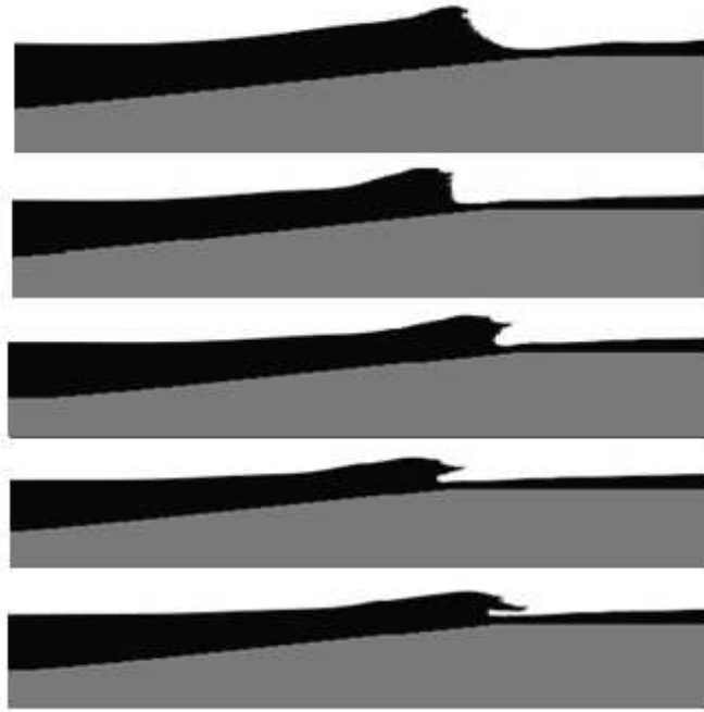
Figure 4.29 - Wave shape on the reef with a submergence of 1.2 m (after 63 s, wave 3).
