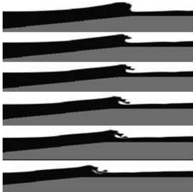
Figure 4.30 - Wave shape on the reef with a submergence of 1.5 m (after 63 s, wave 3).
