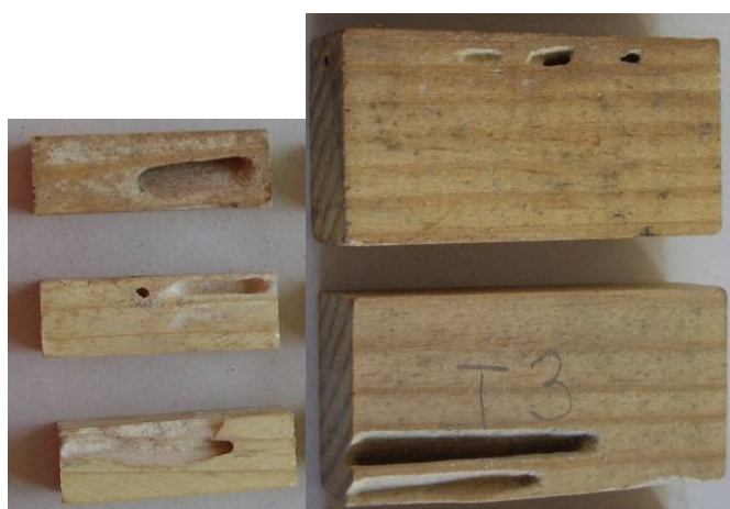
Figure 7: Samples treated with sol-gel after the no-choice test. Left: small specimens; right: EN117 samples
