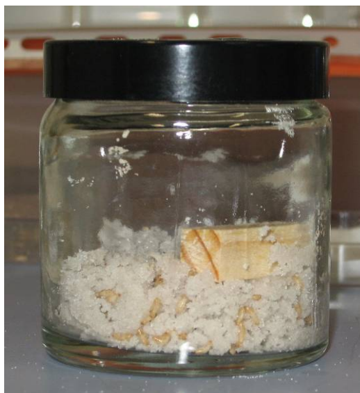
Figure 4: The Reticulitermes grassei no-choice test as adapted from the EN 117 (Nunes 1997)
