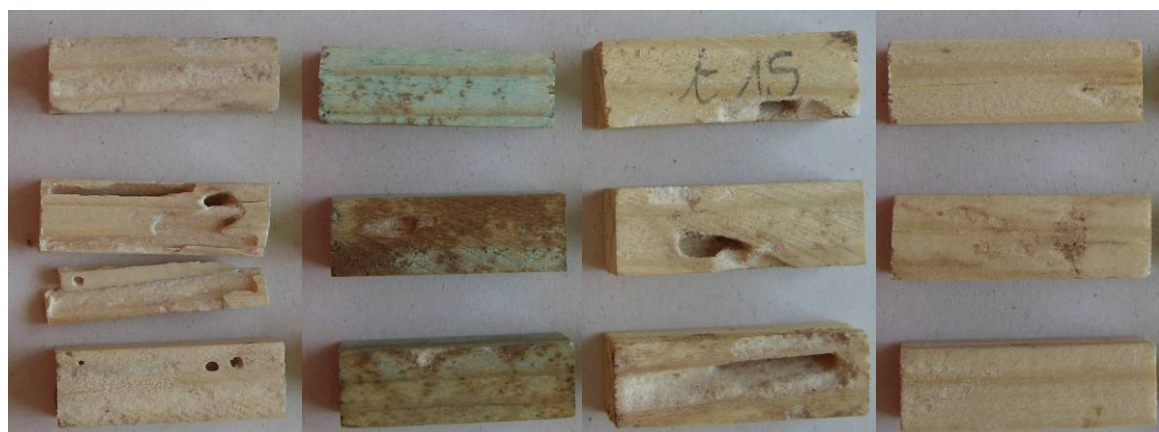
Figure 6: Small samples after the no-choice test. Columns from left to right: controls, sol-gel and copper, sol-gel and boric acid, silicic acid and boric acid treatments
