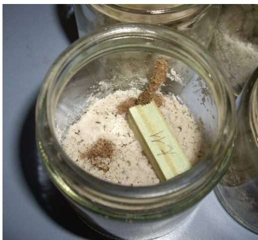
Figure 5: Termites tunnels on a sol-gel and copper treated sample
