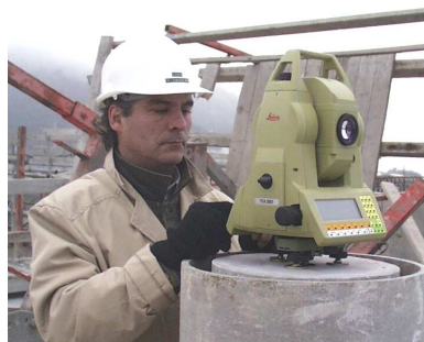
Figure 5 – Tacheometer TCA2003 Figure 6 –Retroreflector GPH1P
