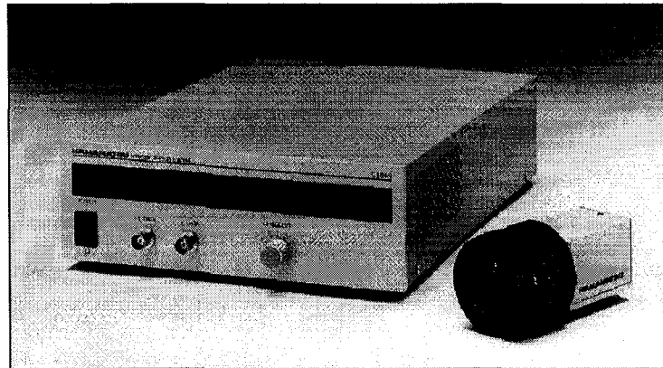
Figure 6: The optical spot position instrumentation unit (C5949 or C2399) using the semiconductor position sensing element (PSD).
