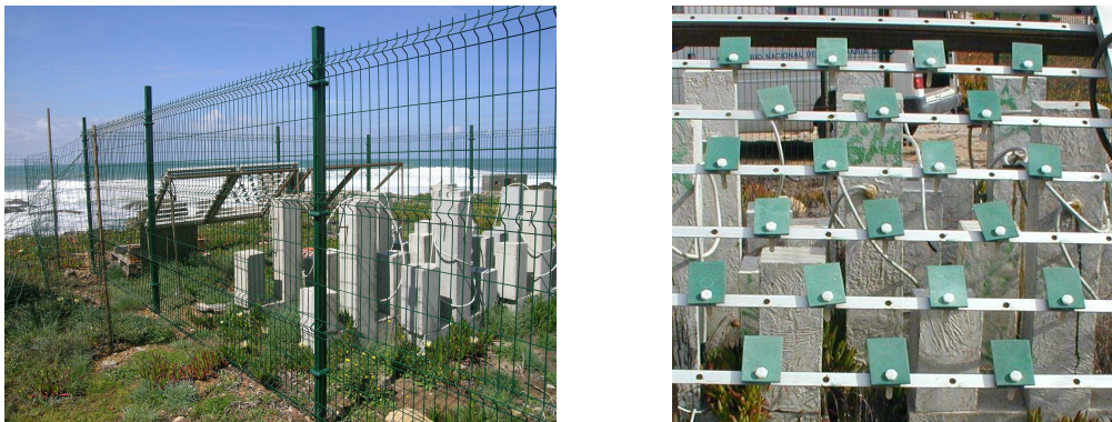
Figure 1 – View of the Cabo Raso test site and visual aspect of all the samples on the exposure rack after 18 months of exposure.
