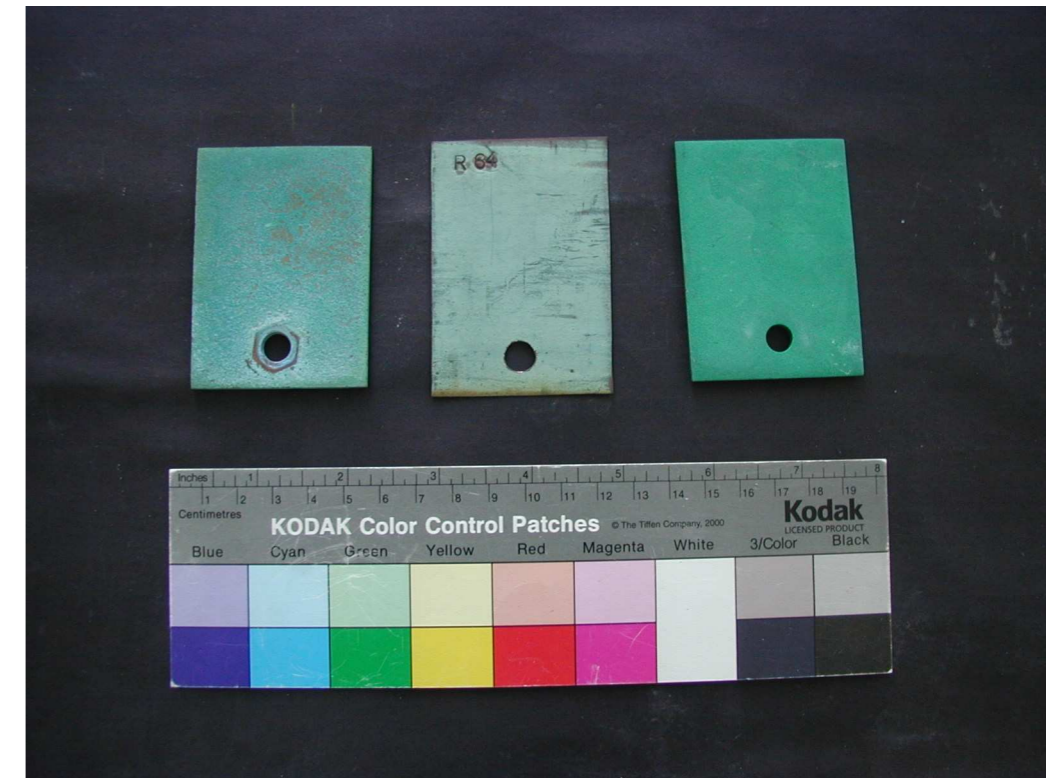
Figure A1 – Visual aspect of MN64, UN(R)64 and UA6 bronze samples before exposure to the salt fog
