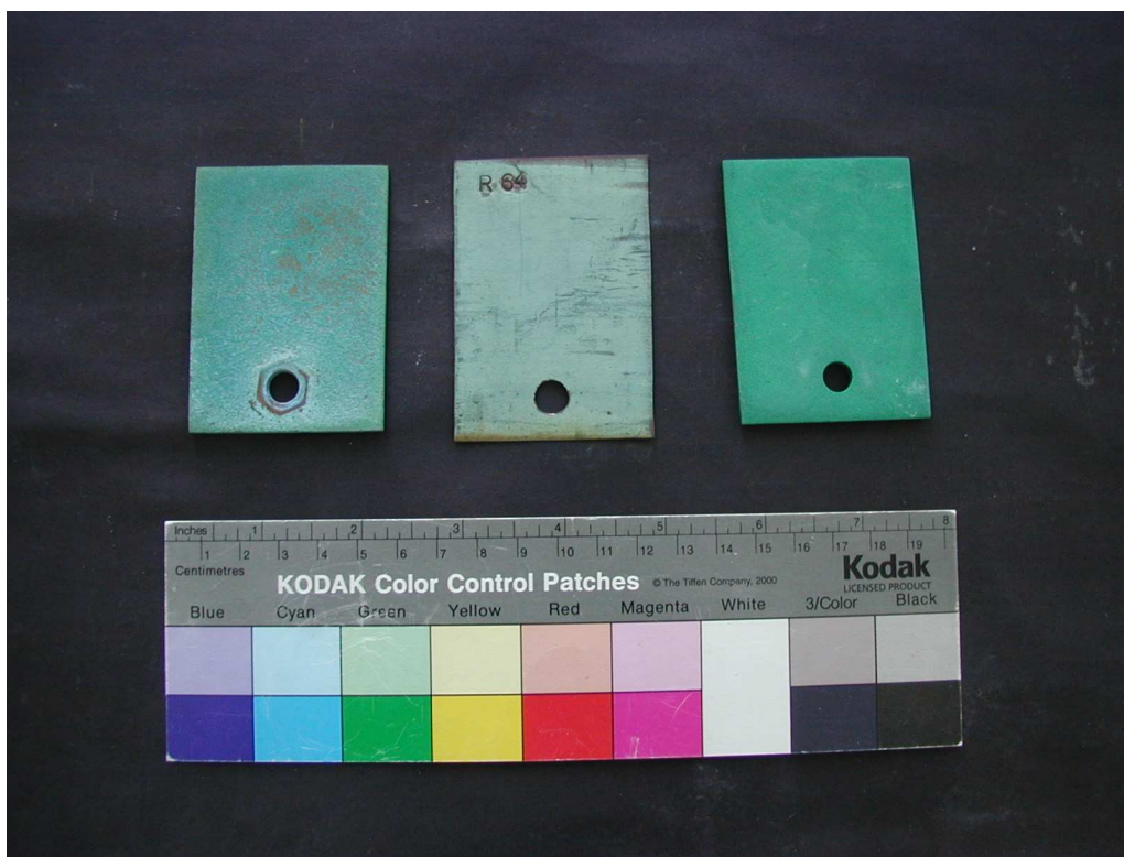
Figure A1 – Visual aspect of MN64, UN(R)64 and UA6 bronze samples before exposure to the salt fog
