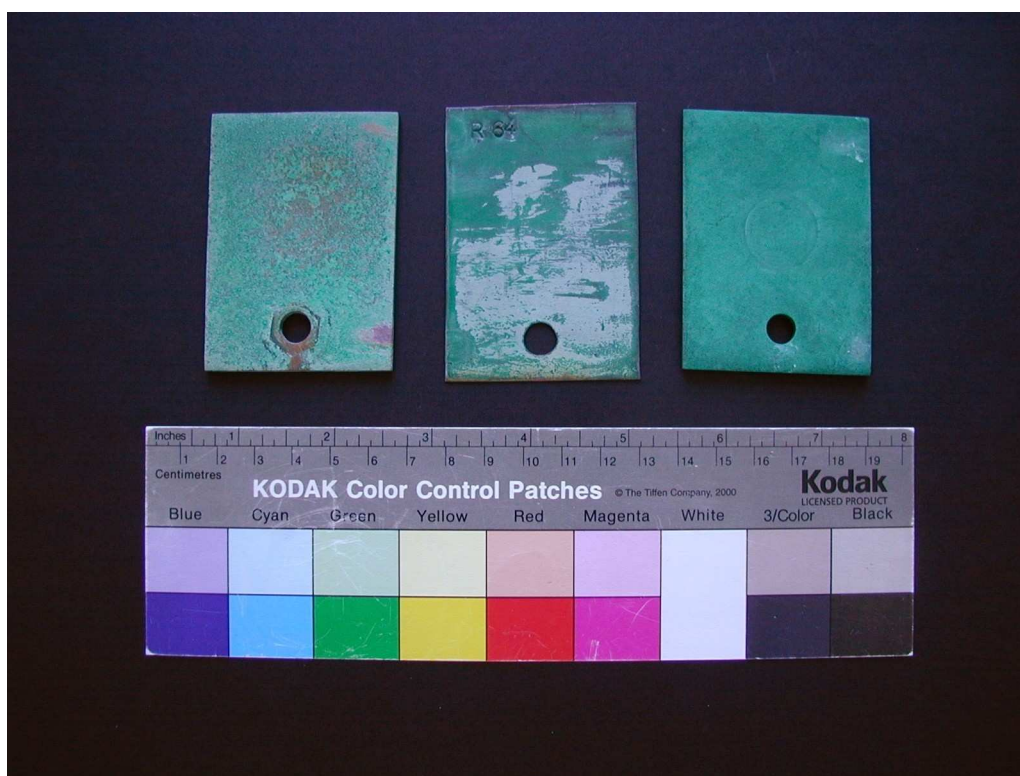
Figure A2 – Visual aspect of MN64, UN(R)64 and UA6 bronze samples after exposure 768 h to the salt fog
