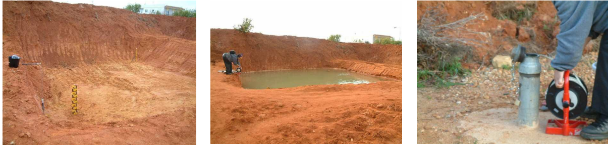
Fig. 3 – Infiltration basin in the second layer and monitoring equipment used for the infiltration test.
