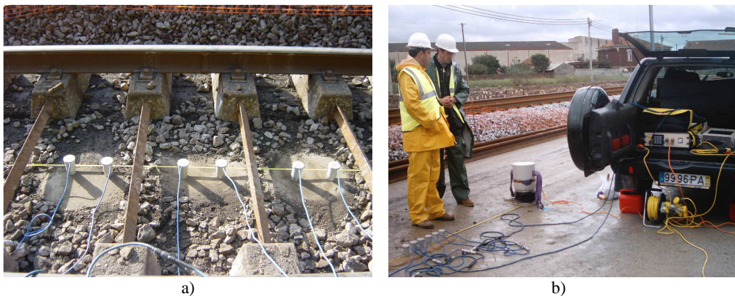
Figure 2. Some aspects of the tests a) SASW on the old platform; b) CSW on the renewed platform.
