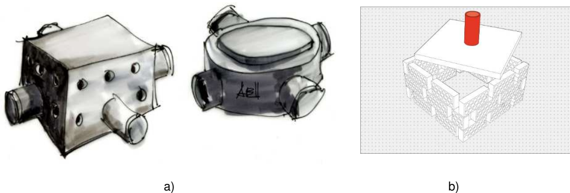
Fig. 5 sumps: a) prefabricated; b) built on site
