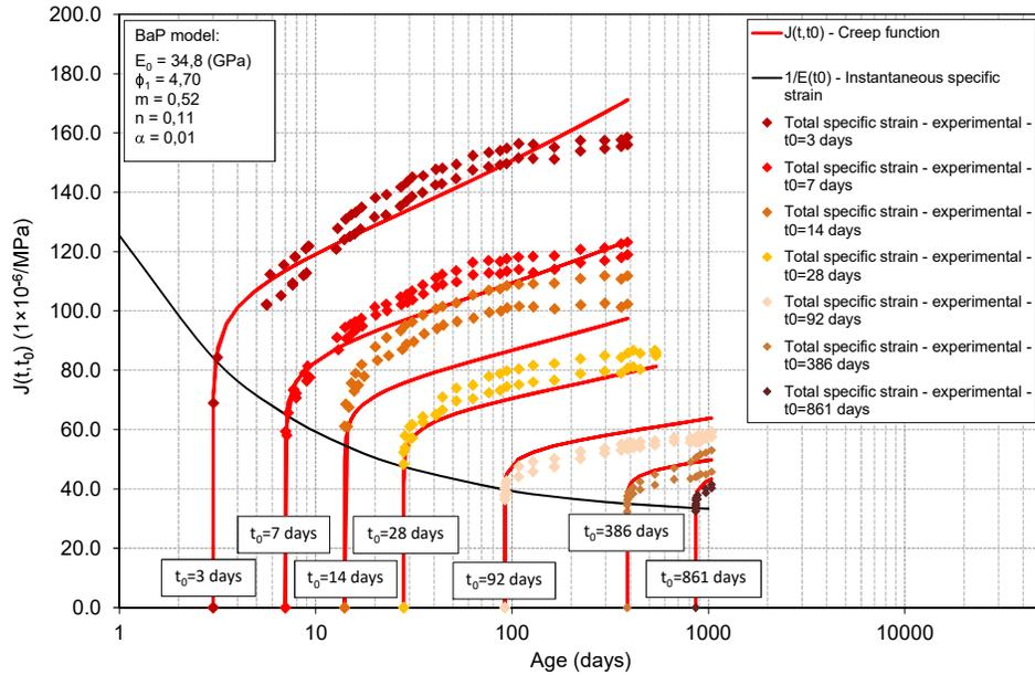
**Fig. 9 – Representation of the creep function fitted from specific strains obtained experimentally for various loading ages**
