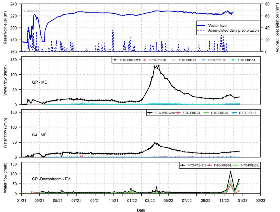
**Fig. 17 – Total flows (drained and infiltrated) observed in weirs located in the drainage gallery, in the radial gallery and in the downstream gallery**
