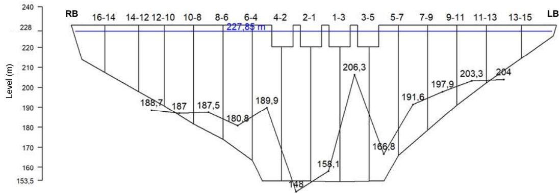
**Fig. 18 – Piezometric elevations corresponding to the uplift observed in the drainage gallery on March 21, 2022, with the reservoir at approximately 228 m**
