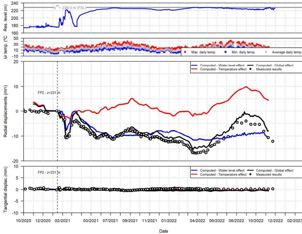
**Fig. 15 – Comparison of the calculated and observed radial and tangential displacements at elevation 231 m on the FP2 plumb line, in block B1**
