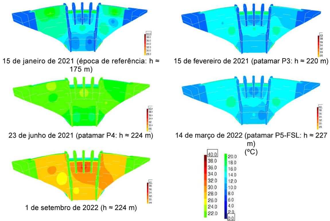
**Fig. 12 – Calculated thermal field in the dam body on different dates during the first filling of the reservoir**
