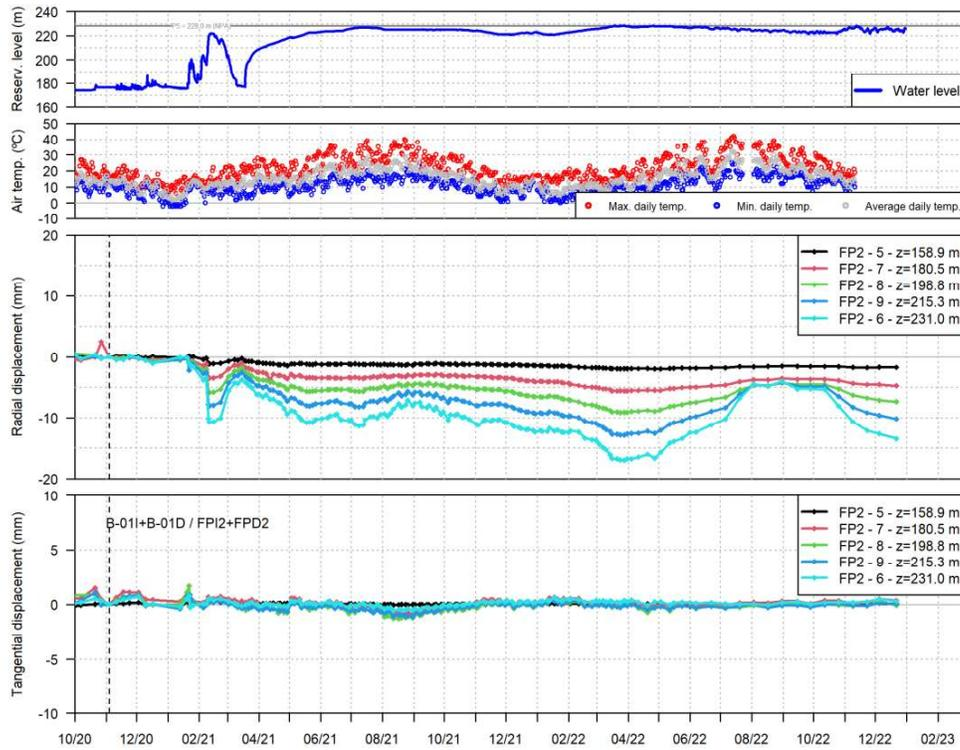
**Fig. 14 – Radial and tangential displacements observed in plumb lines B-01I and B-01D / FPI2 and FPD2, located in block B1**
