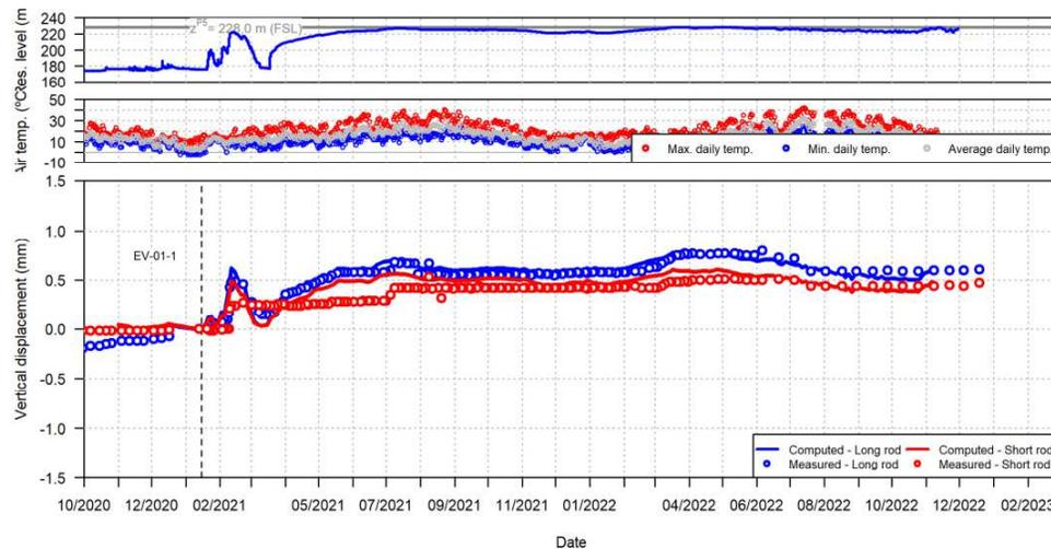
**Fig. 16 – Comparison of vertical displacements calculated with the finite element model and those observed in the rod extensometer EV-01-1, located in the drainage gallery - block B1**
