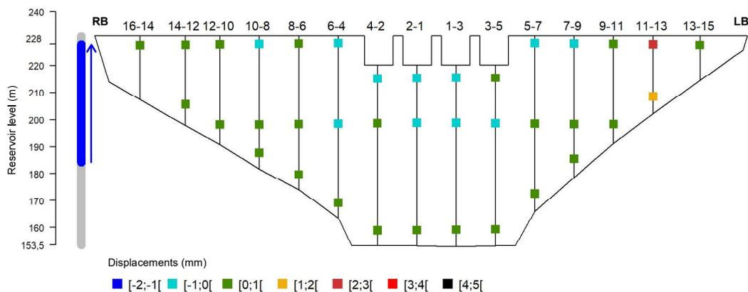
**Fig. 13 – Opening and closing movements observed in 3D surface jointmeters on 03/16/2022 (P5-FSL level, h = 228 m)**
