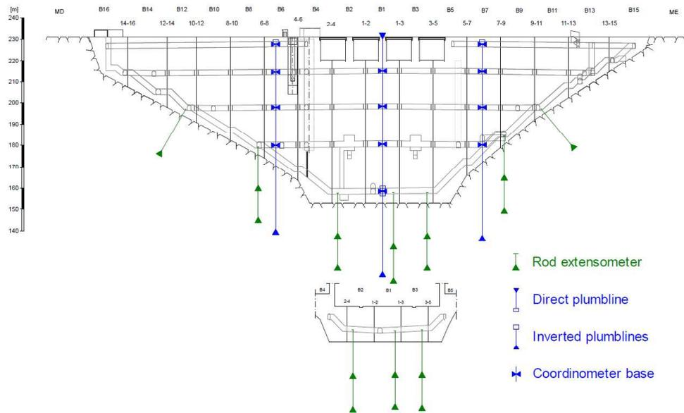
**Fig. 3 – Dam monitoring system – Plumbines and rod extensometers**
