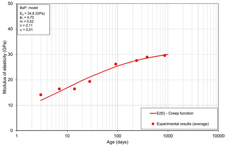
**Fig. 10 – Evolution of modulus of elasticity obtained from experimental tests and from the creep function adopted**
