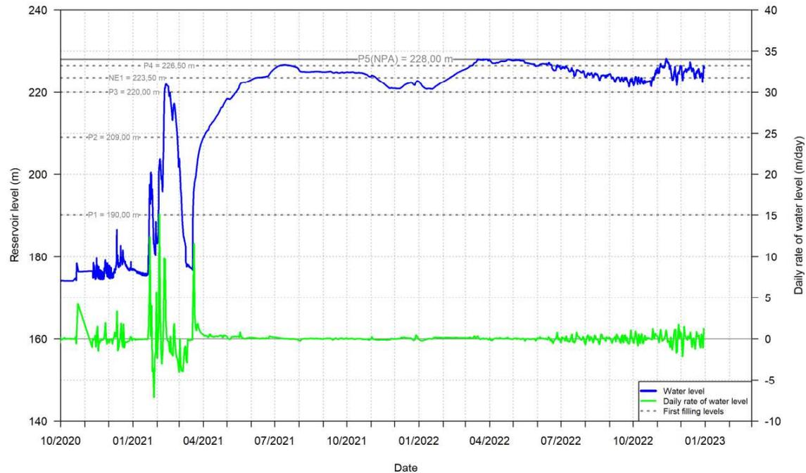
**Fig. 11 – Reservoir level and daily level rate**
