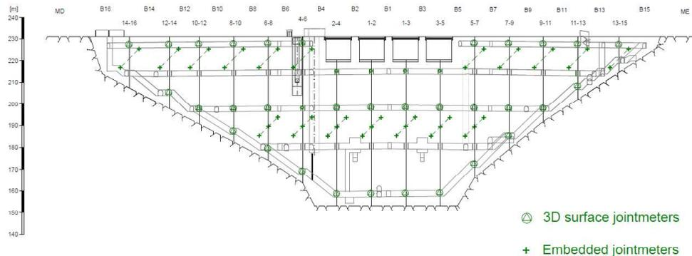
**Fig. 2 – Dam monitoring system – Embedded jointmeters and 3D surface jointmeters**
