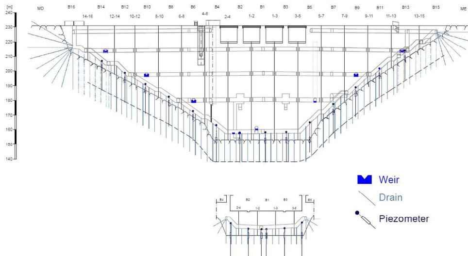
**Fig. 4 – Dam monitoring system – Drainage system and piezometers**
