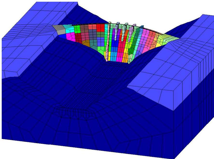
**Fig. 8 – Representation of the finite element mesh of the dam-foundation set, considering the zoning of the dam and the rock mass foundation**
