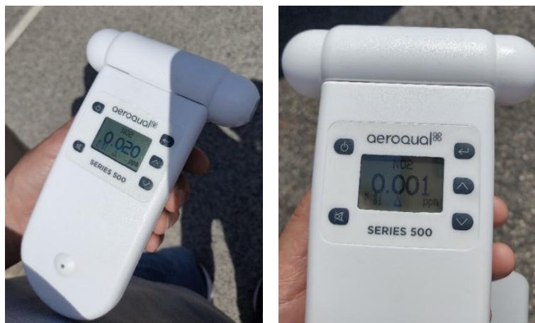
Figure 6.2 – Outdoor nitrogen dioxide measurements at the LNEC campus with the AEROQUAL sensor (29 th July 2023)
