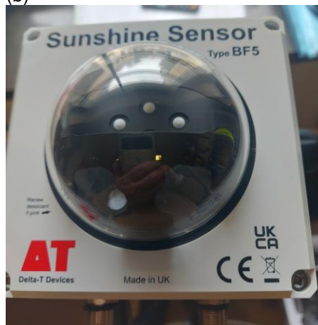
Figure 4.5 – (a) LI-COR illuminance (right) and irradiance (left) sensors on tripods measuring vertical illuminances and irradiances at Ribafria Farm under clear sky conditions and (b) BF5 Sunshine sensor for light and radiation measurements
