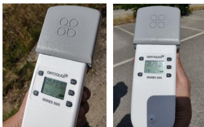
Figure 6.1 – Outdoor particle measurements at the LNEC campus with the AEROQUAL sensor. Differences within short-distance locations were observed, apparently correlated with emission sources (29 th July 2023)
