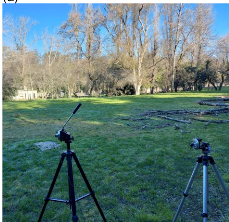
Figure 4.5 – (a) LI-COR illuminance (right) and irradiance (left) sensors on tripods measuring vertical illuminances and irradiances at Ribafria Farm under clear sky conditions and (b) BF5 Sunshine sensor for light and radiation measurements
