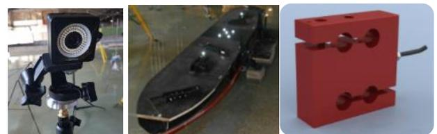
Figure 5. High performance motion capture camera (left). Rigid-body target points array placed on the ship's deck (right). Force sensor.
