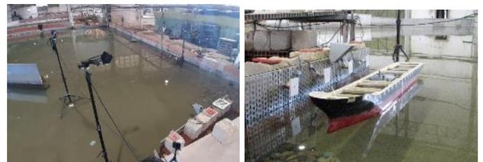
Figure 4. Experimental setup. Ship model and pressure sensors.
