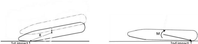
Figure 2. Berthing sequence: 1st impact on the left, 2nd impact on the right.
