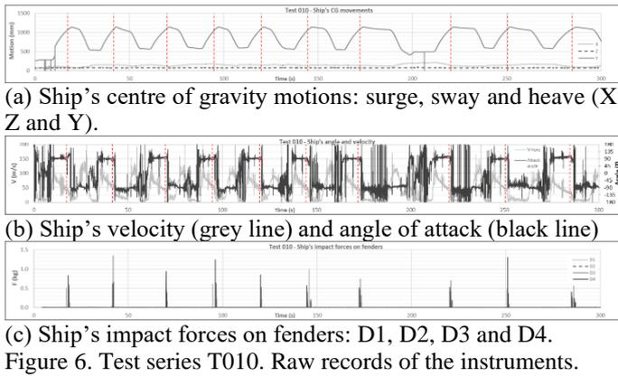
Figure 6. Test series T010. Raw records of the instruments.
