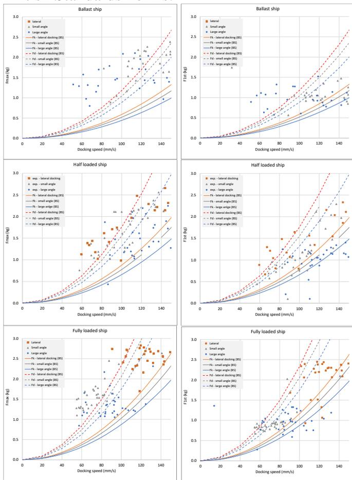
Figure 13. Ship's impact forces on fenders. Comparison of experimental results with British Standards design norms.
