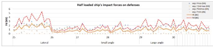
Figure 12.. Comparison of the forces on the 4 fenders,  $F_{max}$ ,  $F_{2nd\ max}$ ,  $F_{3rd\ max}$  and  $F_{min}$ , with Characteristic Force,  $F_k$  and design Force,  $F_d$ , as calculated from BS formulae.
