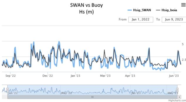
Figure 9. HIDRALERTA EWS validation of wave parameters against wave buoy measurements.
