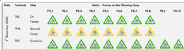
Figure 17. Dashboard of the alerts for the forces on the ships' mooring lines.
