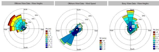
Figure 8 - Offshore (point W) wave (left) and wind (centre) statistics provided by ECMWF. Buoy (B\_PV) measurements wave statistics (right). The dataset encompasses the period from 2005 to 2020.
