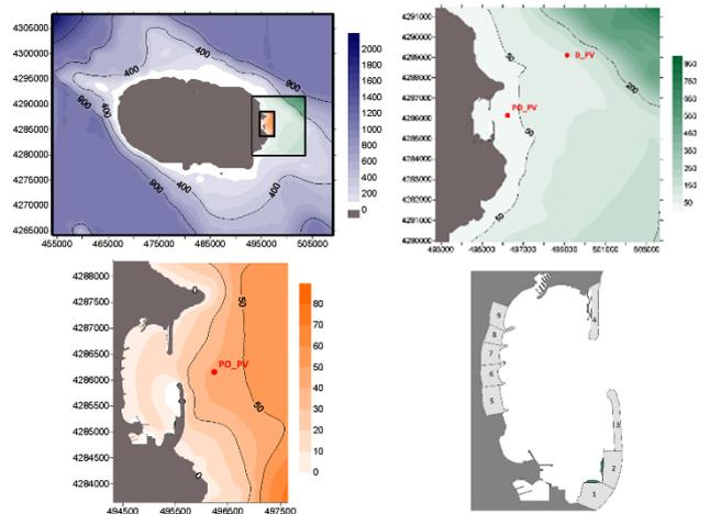
Figure 5. Bathymetry and coarse, medium, and fine grids nested domains for SWAN numerical models. Geographical Location of wave buoys (B\_PV and PO\_PV).
