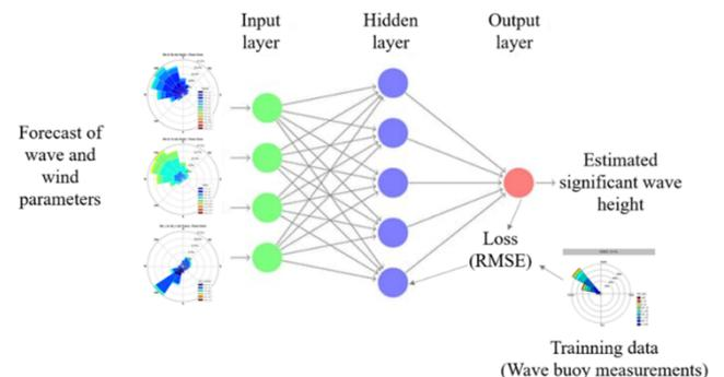
Figure 10 – Structure of the Neural Network for the wave height estimation/forecast at the B\_PV Buoy.
