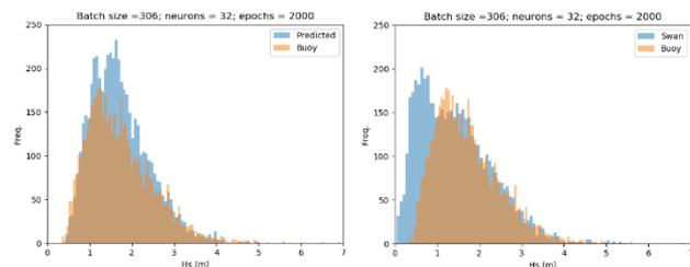
Figure 14 – Comparison of the frequency histograms of Significant wave height Buoy measurements, Neural Network output, and SWAN numerical simulations.
