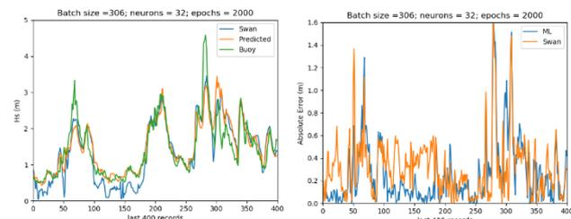
Figure 15 – Comparison of the last 400 records of the Significant wave height Buoy measurements, Neural Network output, and SWAN numerical simulations.
