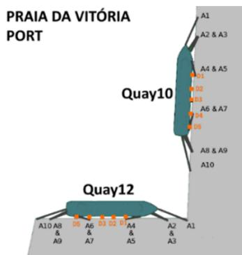
Figure 6. Quay 10 and 12 mooring arrangements for the ships.
