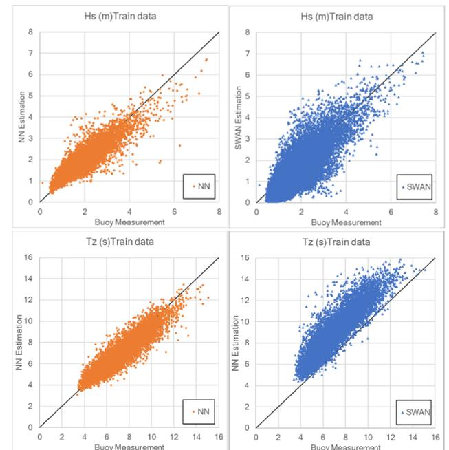
Figure 12 – Significant wave height. Comparison of the NN and SWAN train data. Left: NN; Right: SWAN.
