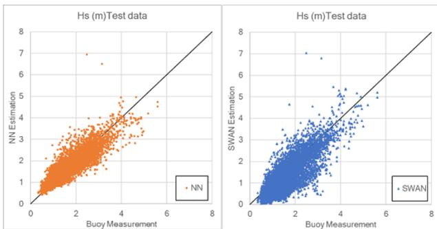
Figure 13 – Significant wave height. Comparison of the NN and SWAN test data. Left: NN; Right: SWAN.
