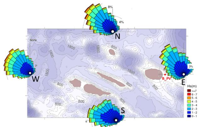
Figure 7. HIDRALERTA EWS four points (N, S, E, W) of offshore wave/wind data used for long-term analysis and as forecast forcing data.
