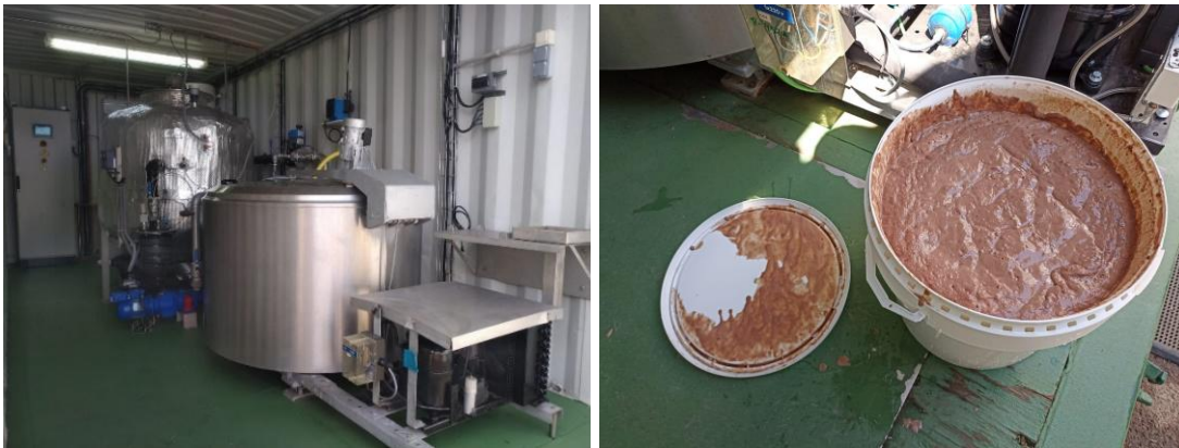
Figure 2: Left: Pilot plant installed in Rincón de León WWTP; Right: Ice cream co-substrate.
