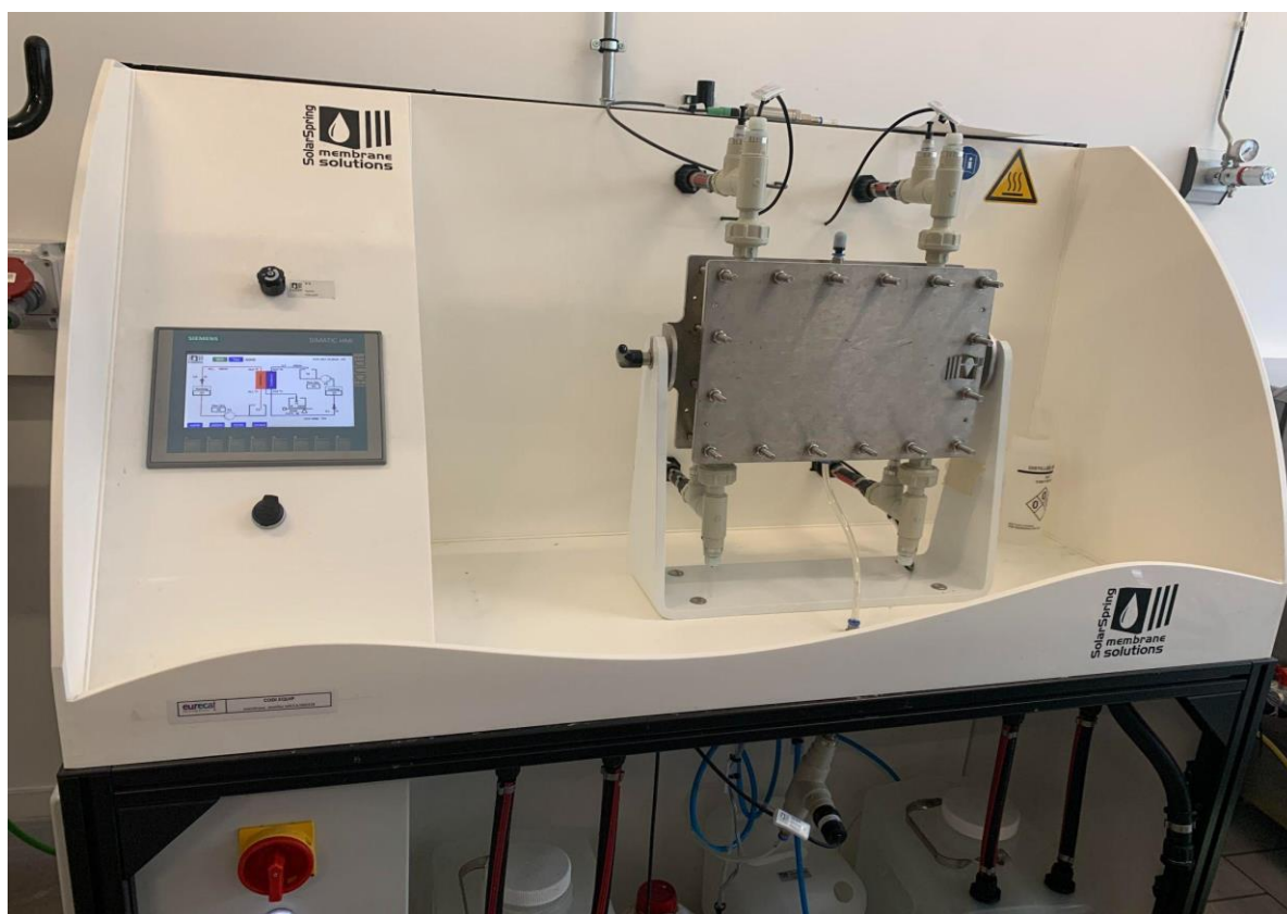
Figure 6: Lab scale SolarSpring GmbH (Germany) membrane distillation (MD) setup at Eurecat (Manresa).
