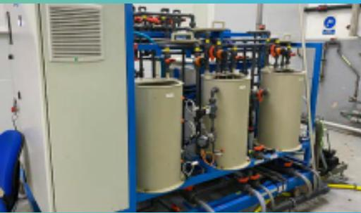
Selective electrodialysis: takes RO brine and separates divalent ions from monovalent ions. The stream with divalent ions will serve as reclaimed water. The stream with monovalent ions will serve as feed for the electrochlorinator
