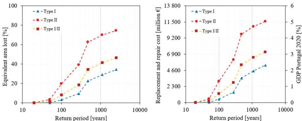
**Figure 12.** Grand total for the pre-code masonry building stock in the MAL region considering different states of conservation/degradation: (a) time-based variation of equivalent area lost; (b) seismic risk curves.
