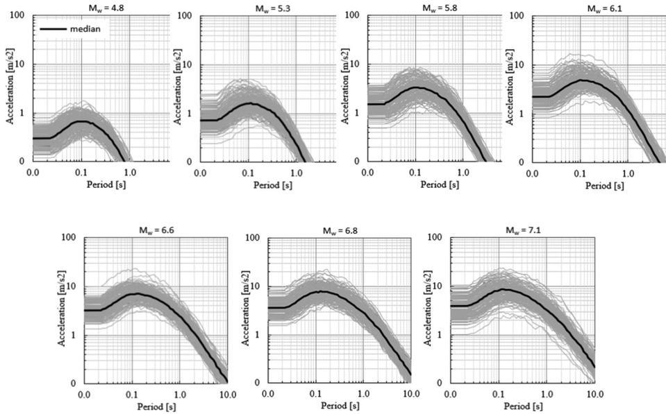
**Figure 4.** Acceleration response spectra at bedrock for LTVF scenario and different magnitudes.
