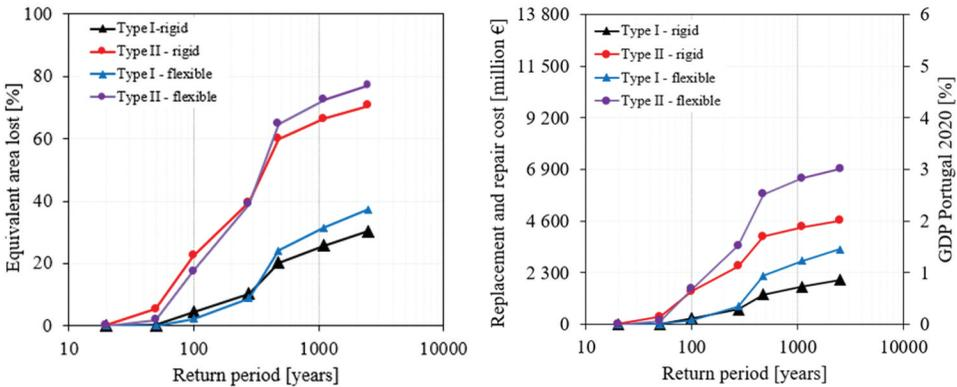
Figure 11. Disaggregation of the losses by typology of pre-code masonry buildings in the MAL region: (a) time-based variation of equivalent area lost; (b) seismic risk curves.
