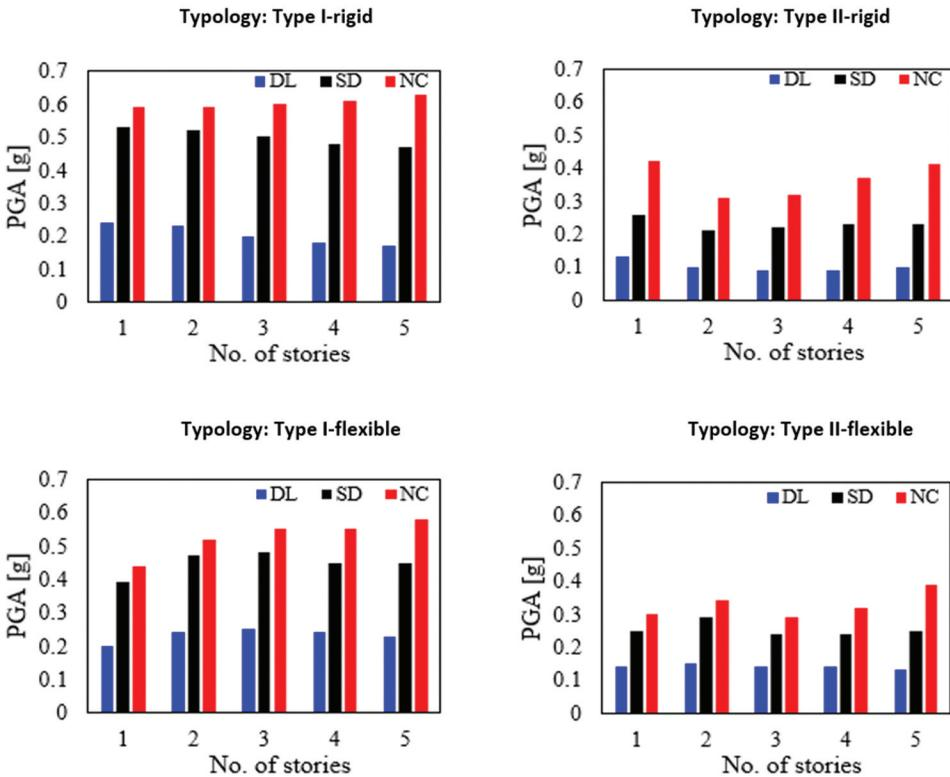
Figure 7. Values of PGA (median quantile) corresponding to the limit state thresholds adopted.
