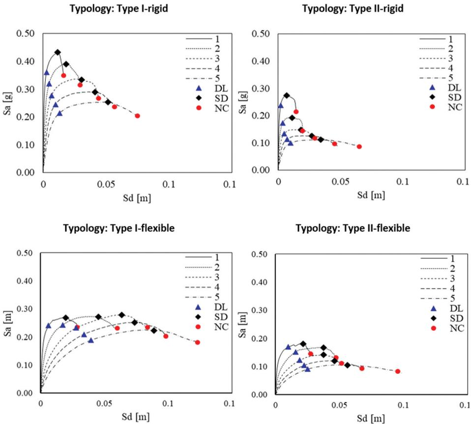
Figure 5. Median capacity curves of the buildings up to five stories high and limit states definition.
