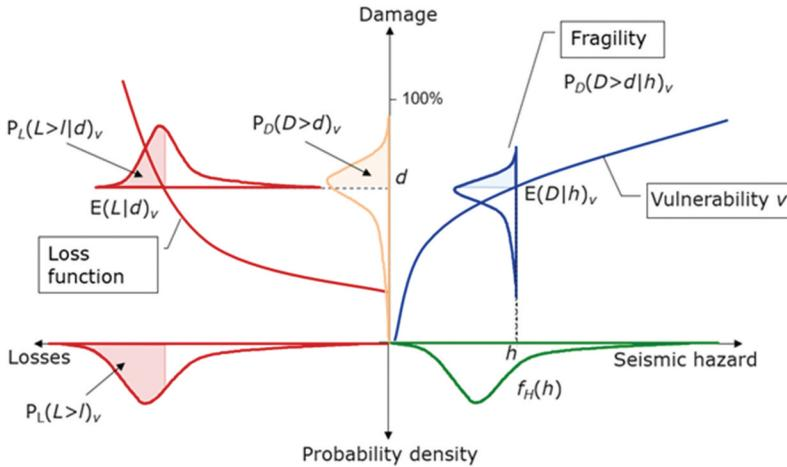
**Figure 1.** Generic scheme of the probabilistic seismic risk modelling for a given structure with vulnerability  $v$  (adapted from Sousa, Campos Costa, and Caldeira 2010).
