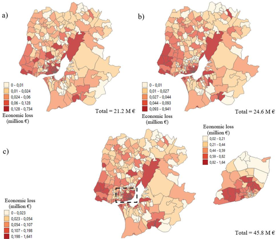
**Figure 13.** Annual expected losses (AEL) of the seismic risk in MAL for pre-code masonry buildings: (a) rigid floors (70% type I + 30% type II); (b) flexible floors (70% type I + 30% type II); (c) grand totals in the MAL region and in the Lisbon city center.
