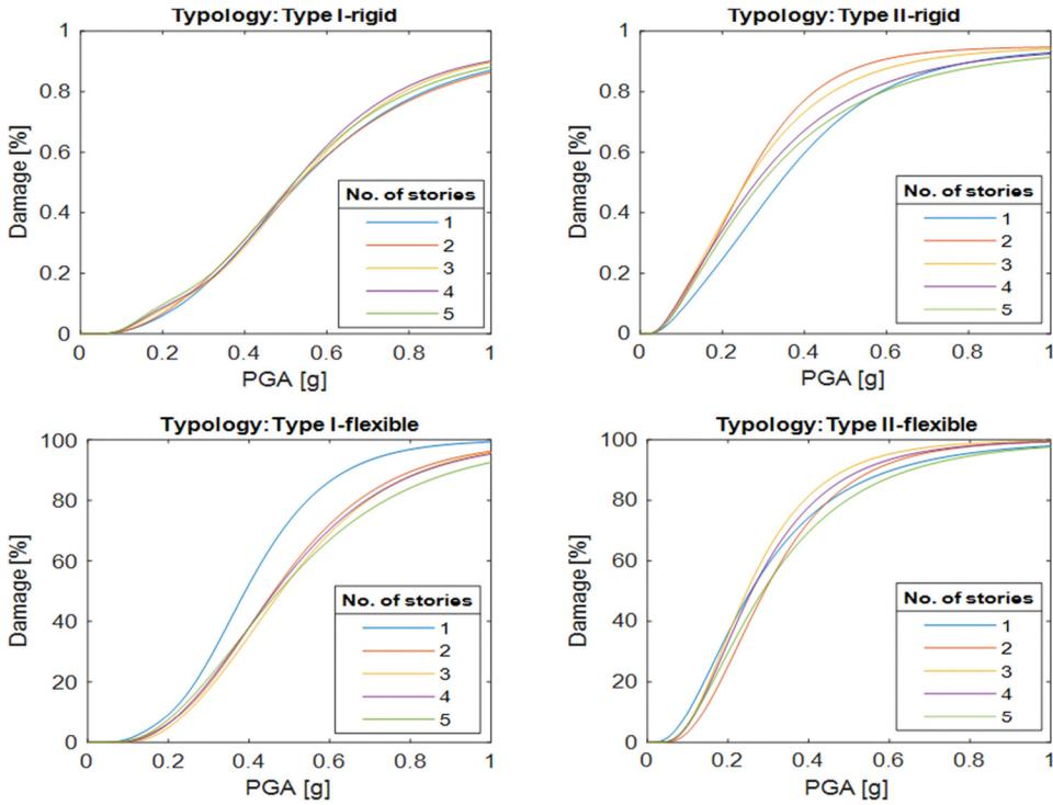
Figure 10. Damage vulnerability functions for different typologies and number of stories.
