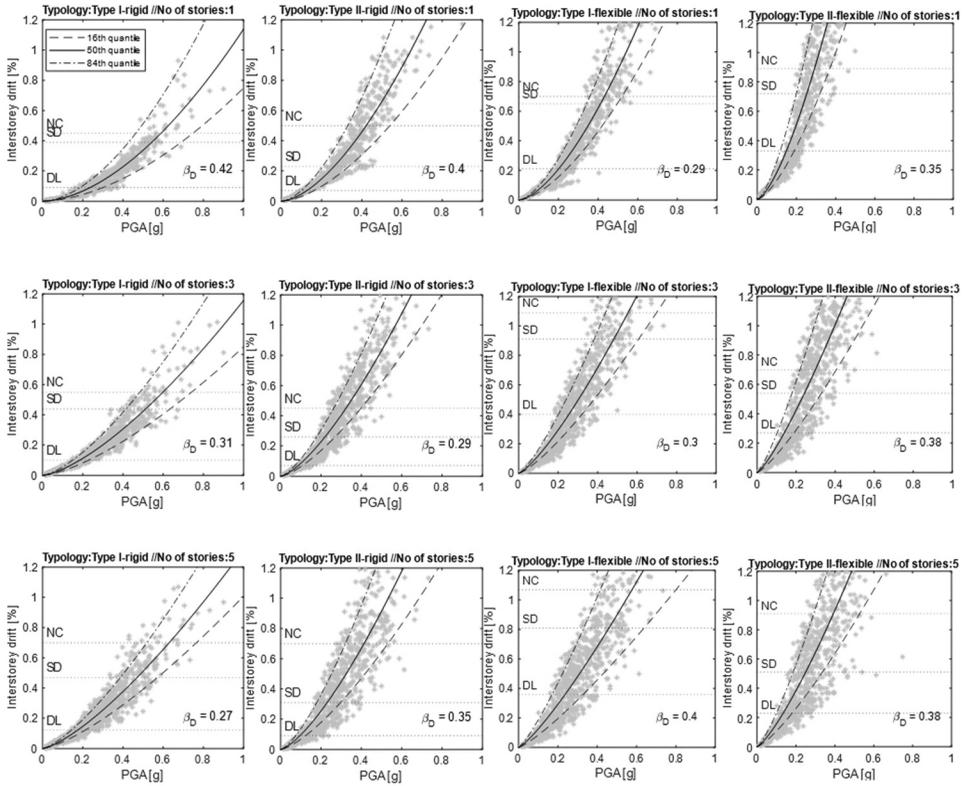
**Figure 6.** Relationship between the interstorey drift (EDP) and PGA (IM); variability in the seismic demand  $\beta_D$ ; definition of the limit states adopted in terms of PGA: DL (damage limitation), SD (significant damage), near collapse (NC).
