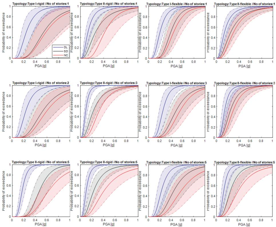
**Figure 9.** Seismic fragility curves for the LS adopted (DL, SD and NC) and buildings with one, three and five stories high (rigid and flexible floors).
