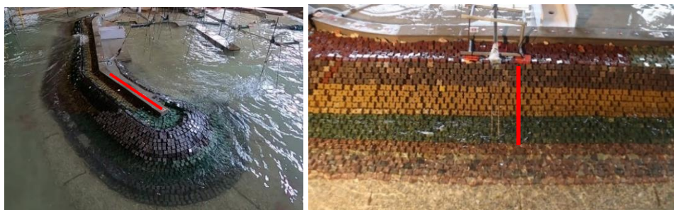
Fig. 1. Three-dimensional model and location of transects (red lines) to retrieve pixel array for Timestack production. Lines are chosen to identify overtopping (left) and run-up events (right).
