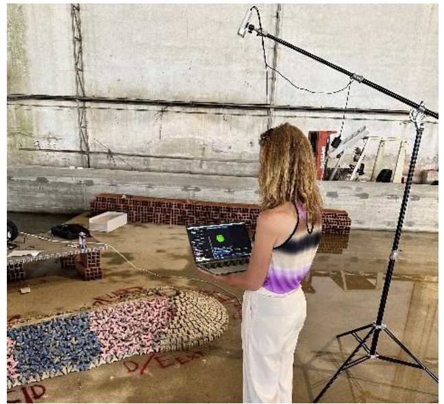
Figure 6. Azure Kinect acquiring and recording 3D model's data.
