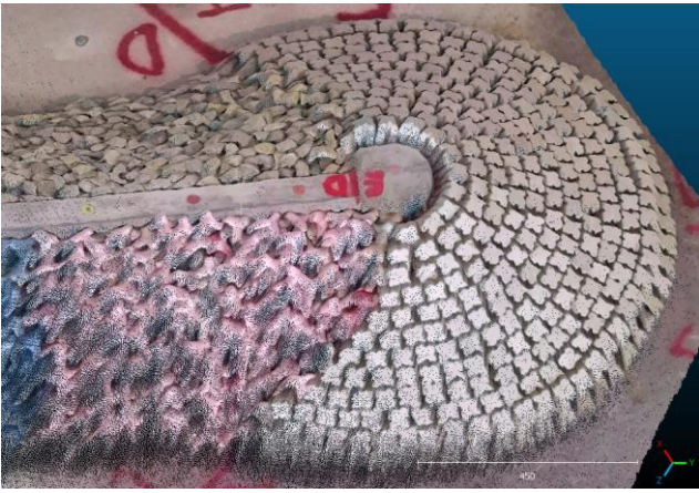
Figure 8. Point cloud obtained with Azure Kinect mkv.
