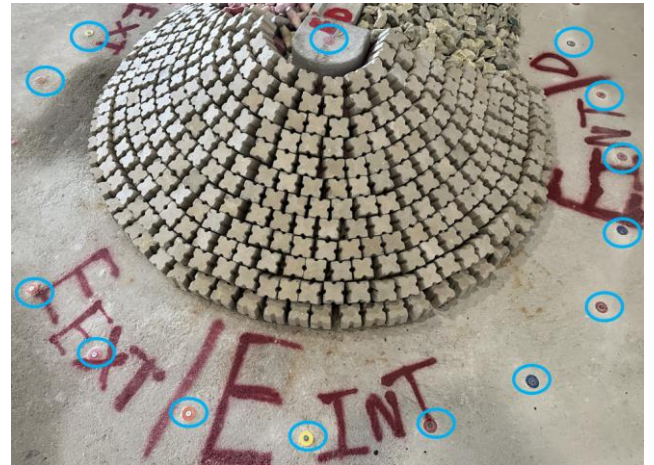
Figure 14. Control points used for georeferencing the point clouds (in blue) and image capture around the model for Photogrammetry and LiDAR techniques.
