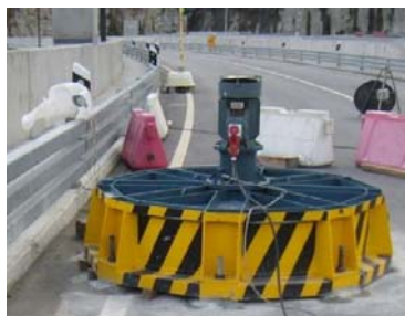
Figure 1. LNEC's eccentric masses vibration generator.
