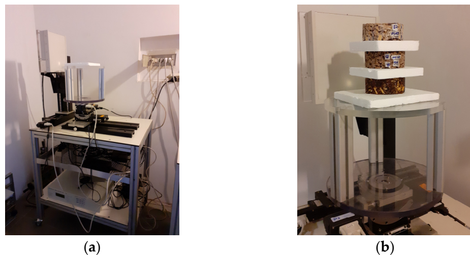
Figure 3. X-ray computed tomography: (a) employed apparatus; (b) three samples separated with expanded polystyrene boards placed on the rotation platform.
