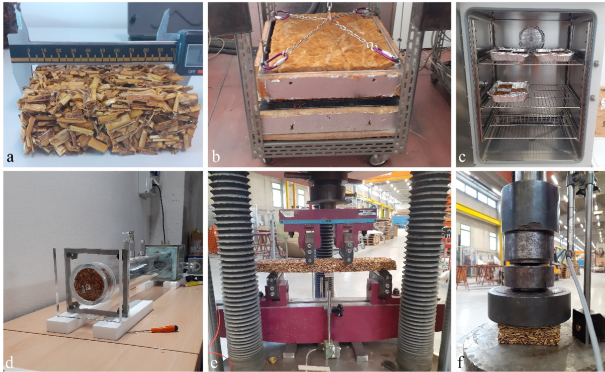
Fig. 3. Main tests of the experimental campaign: a) evaluation of the apparent density of a giant reed-based composite sample; b) equipment to evaluate the thermal conductivity by the heat flow method; c) composite samples into the climate chamber during the hygroscopicity test; d) a cylindrical sample of giant reed into the impedance tube to evaluate the sound absorption capacity; e) giant reed-based sample (10 cm x 50 cm x 4 cm) in the Galdabini machine at the beginning of the bending test; f) giant reed-based sample (10 cm x 10 cm x 4 cm) before the performance of the compressive test.
