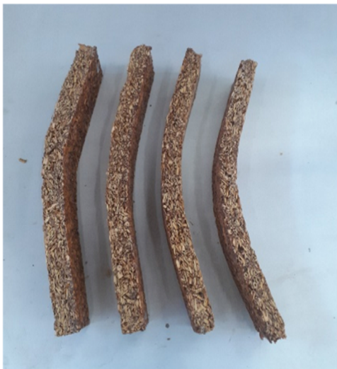
Fig. 7. Four samples (10 cm \times 50 cm \times 4 cm) of giant reed and sodium silicate solution after the bending test.
