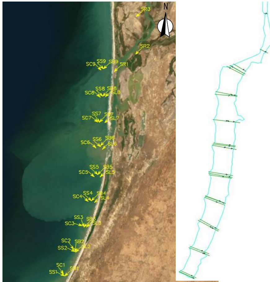
Figure 2.4 – Location of the sediment samples collected in the sedimentological campaign of January 2019 in the coastal area of Saint-Louis, Senegal; schematic layout of the cross-shore profiles extracted from the DTM developed in this study that contain the position of the sediment samples
