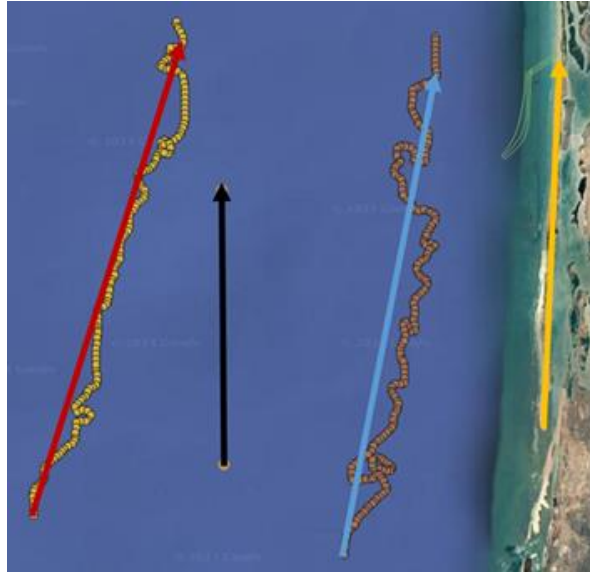
Figure 2.3 – Vectors indicating the coastline and foreshore orientations at 0 m (yellow arrow), 20 m (blue arrow) and 50 m (red arrow) isobaths; the black arrow stands for the geographical “true” north orientation ( -0.45^\circ in the study reference system)
