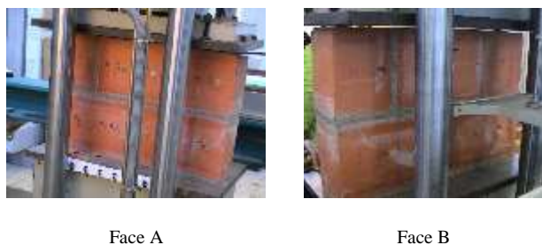
Fig. 6: The phase of preparation of Specimen A1 for the compression test (view of the face A and B of the specimen)
