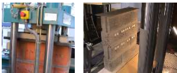
a) Specimen A1 (perforated ceramic blocks) b) Specimen A2 (massive concrete blocks of expanded clay aggregates)
