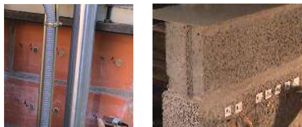
a) Specimen A1 (perforated ceramic blocks) b) Specimen A2 (massive concrete blocks of expanded clay aggregates)
