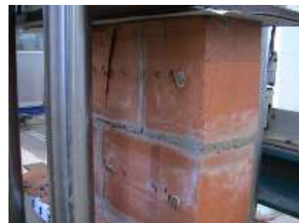
Fig. 10: Aspect of the face A of Specimen A1 at the end of the test after discharge of a load of 470 kN
