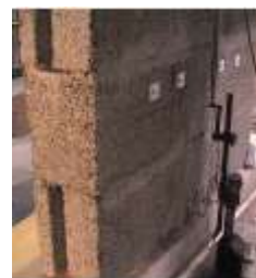
Fig. 17: Aspect of the face B of Specimen A2 at the end of the test, with evident signs of local fragmentation of the base of specimen
