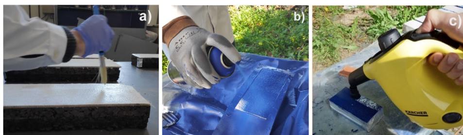
Fig. 1 a Application of anti-graffiti products; b application of aerosol paints (ultramarine blue); c removal of graffiti with a low-pressure steam jet and brushing
