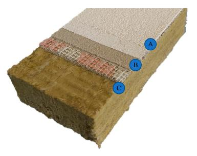
**Figure 1.** Example of an external thermal insulation composite system (ETICS), in which (**A**) is the finishing coat, (**B**) is the base coat with reinforcement mesh incorporated between the layers and (**C**) is the thermal insulation (in this case MW).
