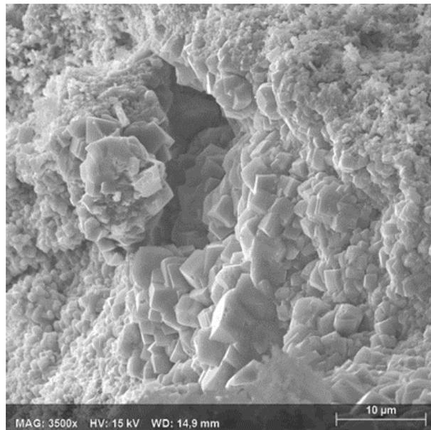
**Figure 14.** SEM image with a magnification of the 3500x and a working distance (WD) of 14.9 mm at A+Q30%:M<sub>2</sub> mortar where it is possible to observe the large capillary pores filled by carbonate crystals after cycles.
