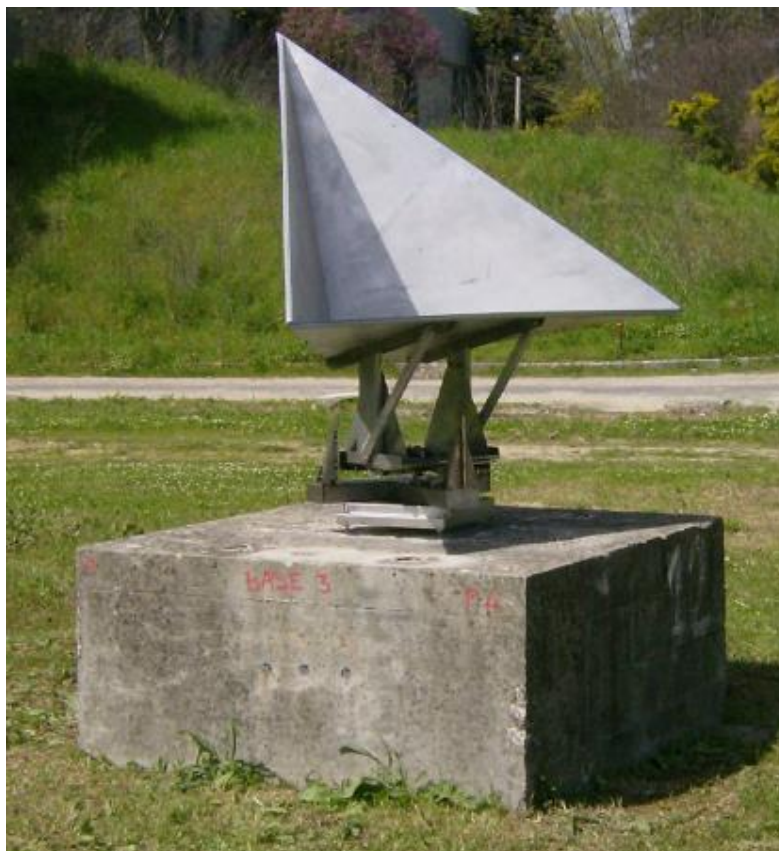
Figure 107 – Individual CR of the triangular trihedral model oriented towards the LOS of the descending pass.
