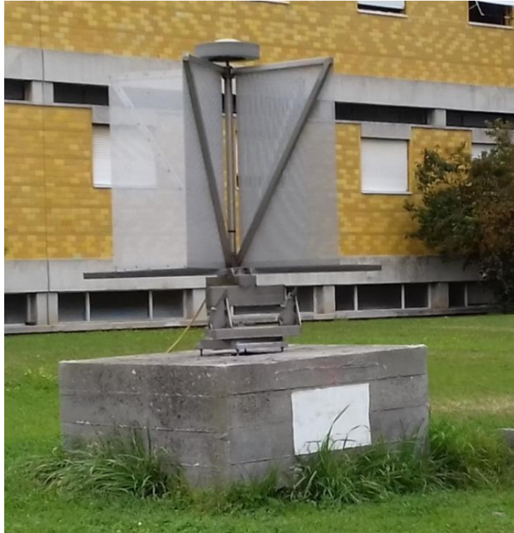
Figure 104 – Bidirectional corner reflector proposed in this study.
