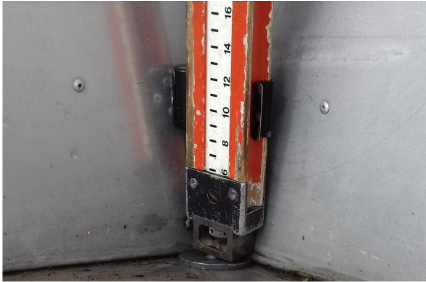
Figure 112 – Levelling rod at the centre of triangular trihedral with the aid of a metallic piece.
