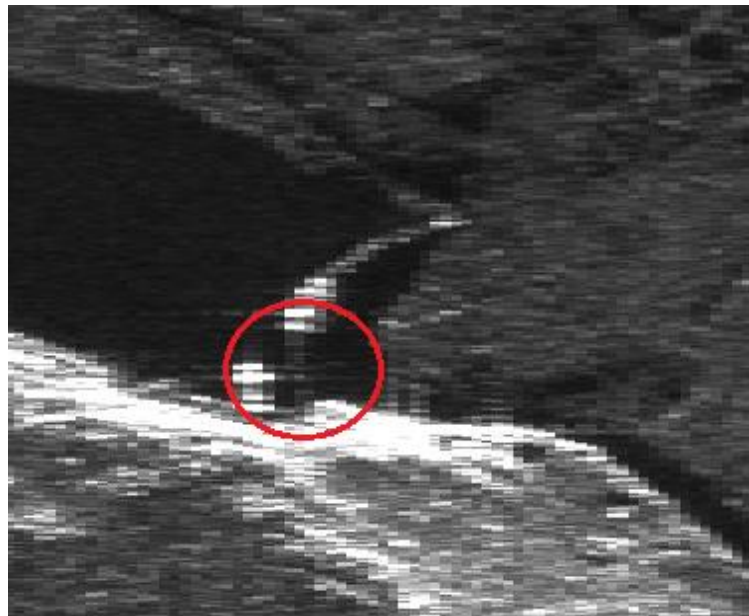
Figure 96 – Reflectivity map of the dam from the descending pass acquisition geometry; red circumference highlights the zone in the dam crest with gaps in PS acquisition and low reflectivity.
