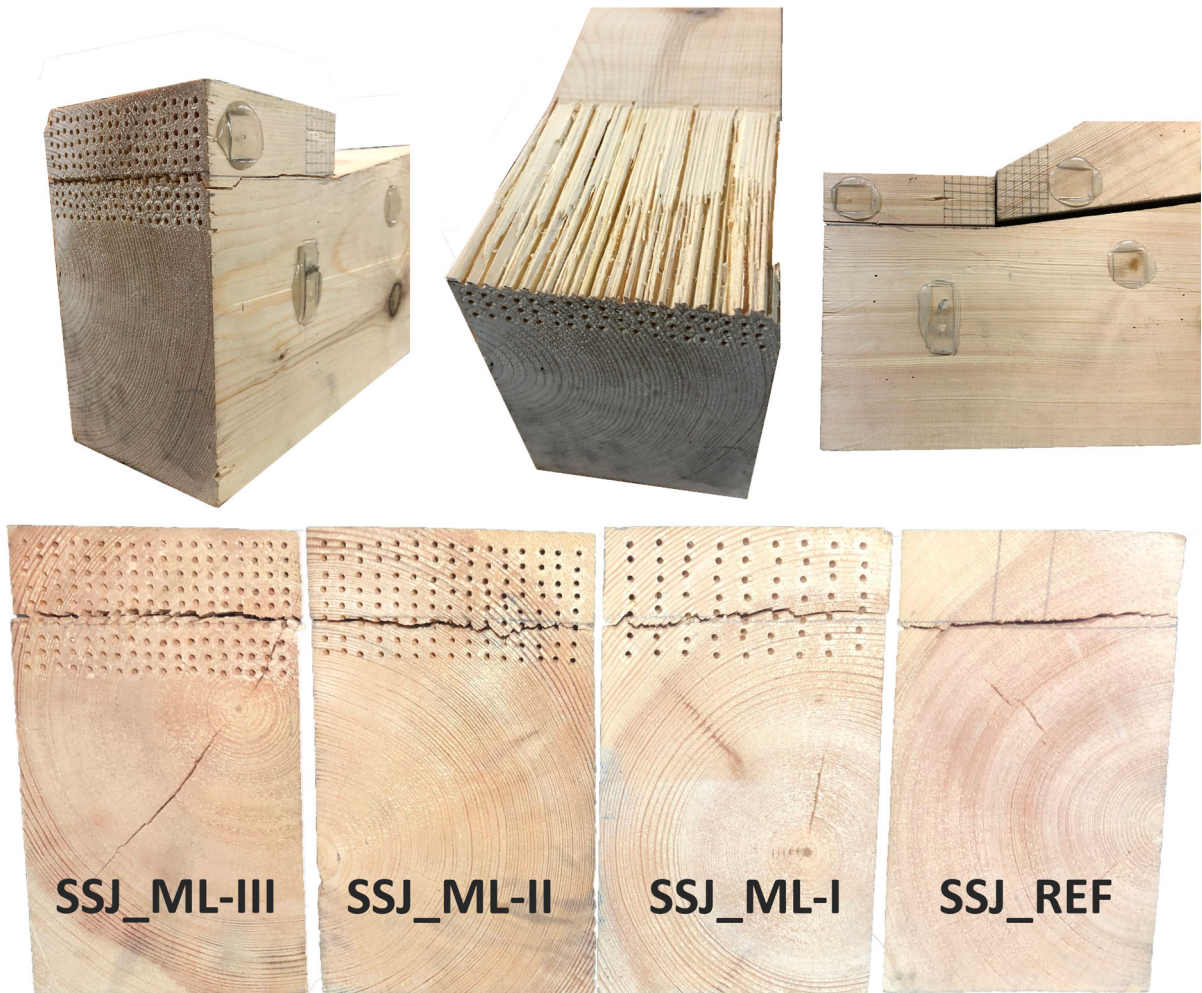
Fig. 5 Characteristic shear failure on the tie beam-end observed in all Single Step Joints tested under compression
