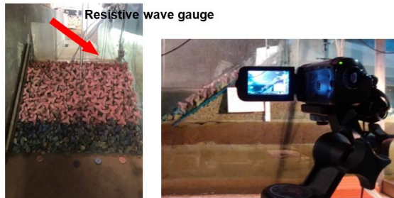
Figure 4. a) Resistive wave gauge b) video camera outside the flume
