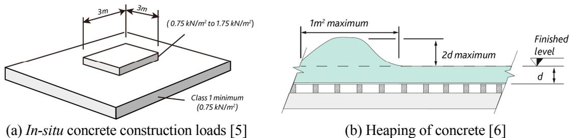
**Fig. 3:** Casting construction loads
