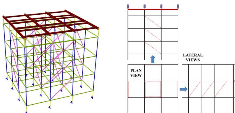
**Fig. 2:** Structural layout of Model A2
