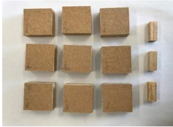
Figure 3.1 – Aspect of AGEPAN® DWD PROTECT samples (n=9; at left) and maritime pine (n=3, at right) at the end of the test of resistance to moulds
