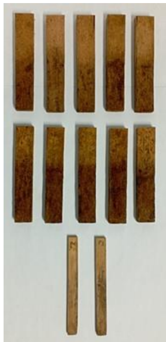
Figure 3.2 – Aspect of the samples of AGEPAN® DWD PROTECT (first row), AGEPAN® DWD PROTECT submitted to leaching (second row), and maritime pine (third row), at the end of the soft rot test of 12 weeks of exposure time
