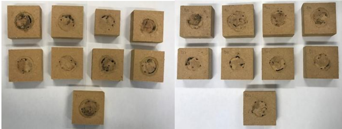
Figure 3.6 – Durability against subterranean termites: Aspect of the AGEPAN® DWD PROTECT samples (left image), and of the AGEPAN® DWD PROTECT samples submitted to leaching (right image) after the test adapted from EN118 (2013)
