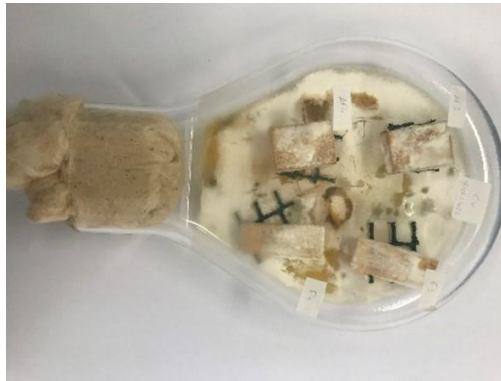
Figure 2.2 – Durability against wood rotting fungi (miniblocks): example with exposure to C. versicolor
