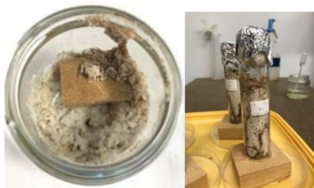
Figure 2.4 – Durability against subterranean termites: Examples of the exposure conditions of the test adapted from EN117 (2012; left) and of the test according to EN118 (2013; right)
