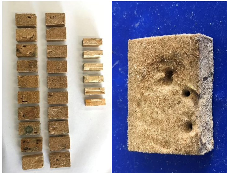
Figure 3.4 – Durability against subterranean termites: Aspect of the tested specimens - AGEPAN® DWD PROTECT samples in the first column, AGEPAN® DWD PROTECT samples submitted to leaching in the second column, and maritime pine in the third column (left image), and example of one sample of AGEPAN® DWD PROTECT submitted to leaching (right image) after the test adapted from EN117 (2012) showing extensive tunneling by the termites
