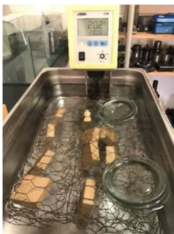
Figure 2.1 – Swelling in thickness test. Samples under immersion
