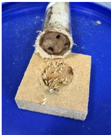
Figure 3.5 – Durability against subterranean termites: Aspect of the end of the test adapted from EN118 (2013) with an AGEPAN® DWD PROTECT sample, and the termites installed in the sample
