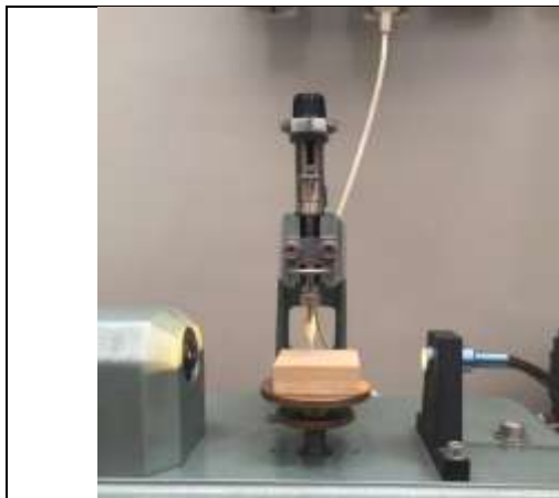
Fig. 9. Apparatus for the measurement of contact angle
