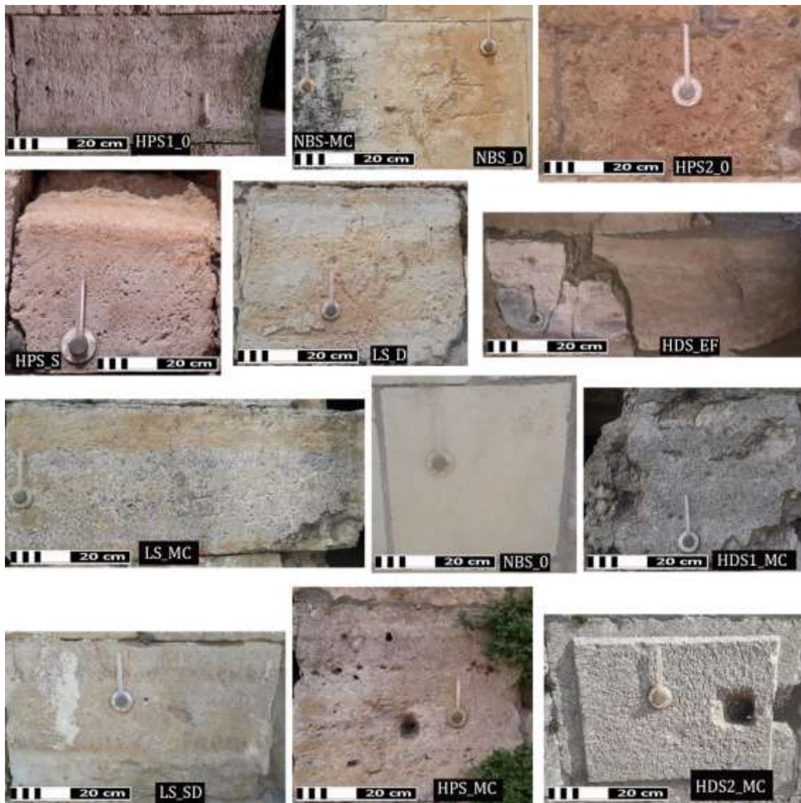
Figure 9 the tested stones by Rilem tube and Schmidt hammer.
