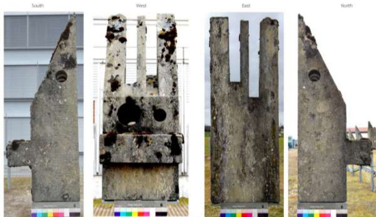
Figure 4. Asterix No 9 (non-consolidated) in 2019, from left to right: sides exposed to South (Alps), West, East and North. The East side shows a differentiated soiling pattern following the two different water run-off regimes facilitated by the different geometries of the incisions where the one on the left (southward) slopes towards West and the one on the right has a horizontal base.
