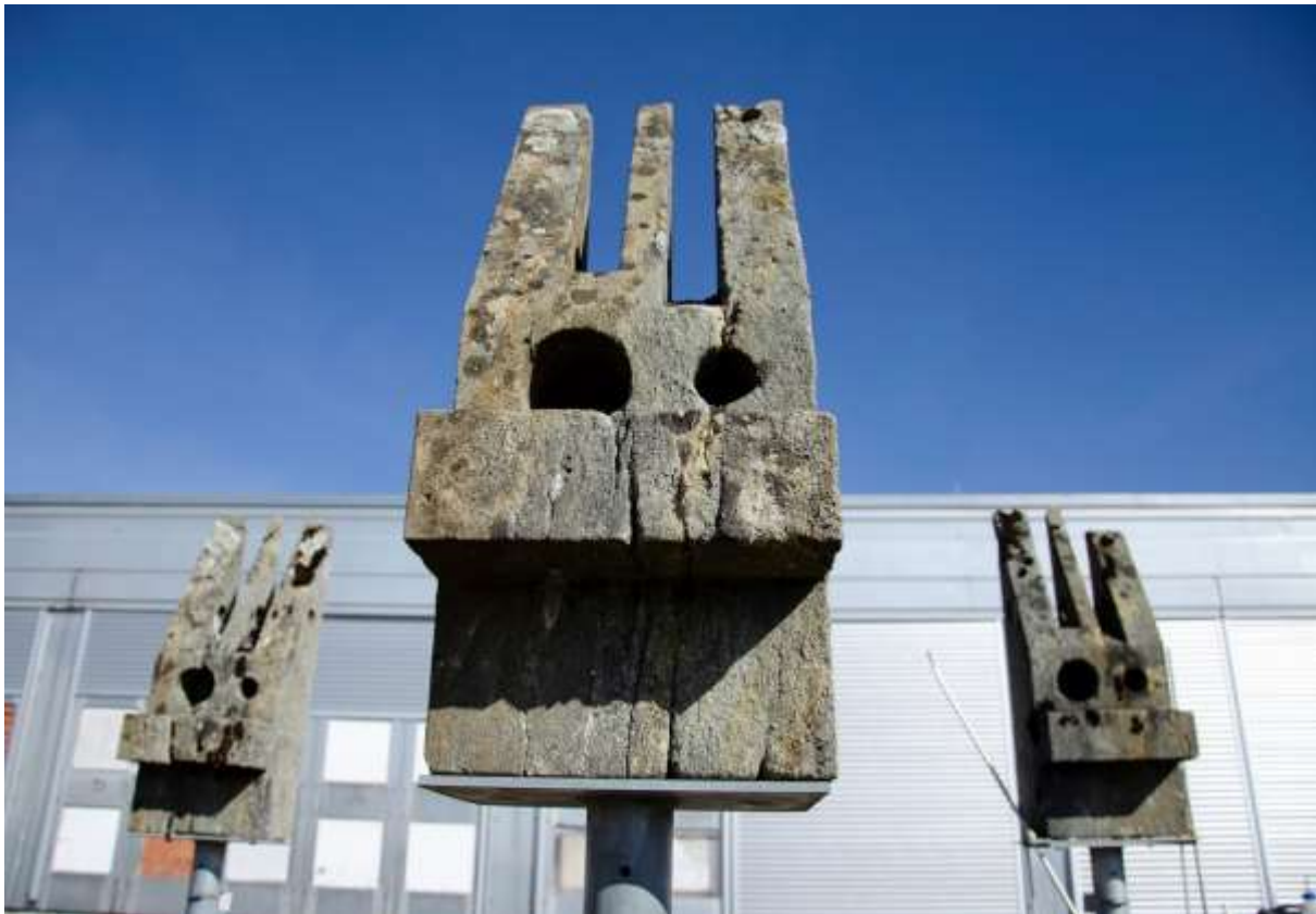
Figure 1. Holzkirchen (Germany) March 2019, outdoor test site with a selection of Asterixe specimen with the front facing West and the South side facing the Alps (middle foreground: Asterix No 4 was part of this study; ©Wilhelm 2019).
