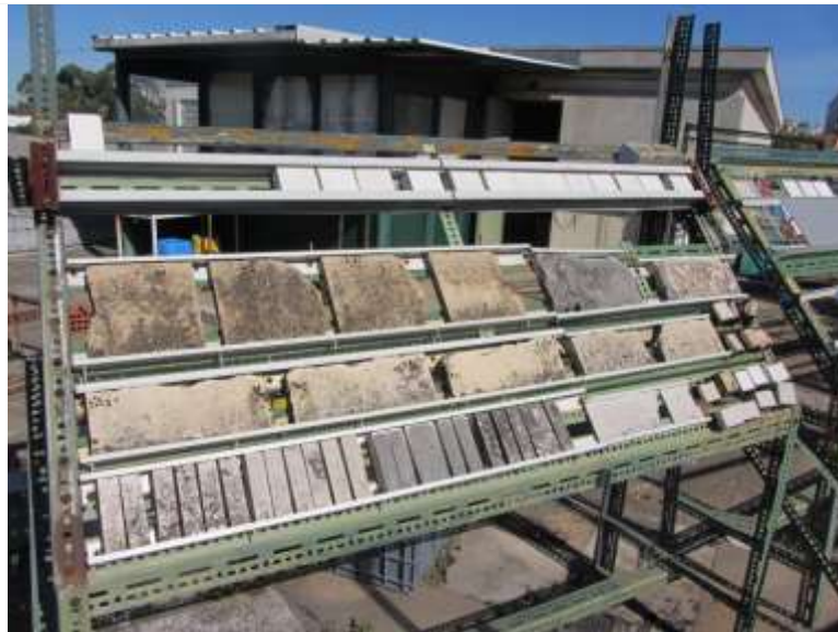
Fig. 4 – Example of outdoor exposure trial arrangements showing specimens of different sizes and shapes.
