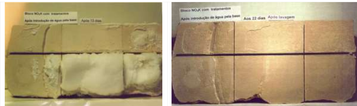
Figure 6 – Aspect of the AS block (28% porosity) treated with different products after forced percolation of a salt solution (left) and after removal of efflorescences (right). The central test area in the bottom row showing an intense salt blossoming is the zone treated with ethyl silicate. The central test area in the upper row was treated with Paraloid B72. The block is about 35 cm long
