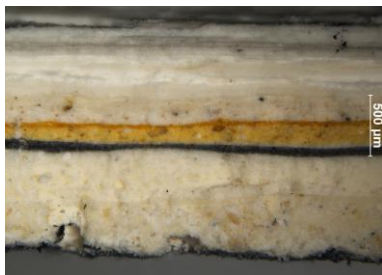
Figure 1. Unpolished cross section from the wall painting covering layer, Magleby Church Denmark. From the bottom, the contact surface with the original wall painting and towards the top of the picture still newer added layers.
