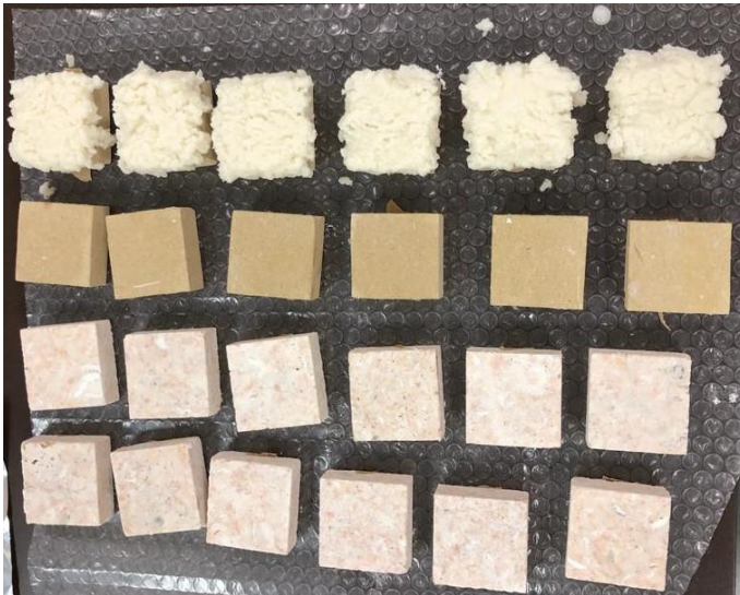
Fig. 1. Treated samples. The image shows the stone samples during the application of DAP. In particular, the upper row shows the Finale stone samples with the poultice.
