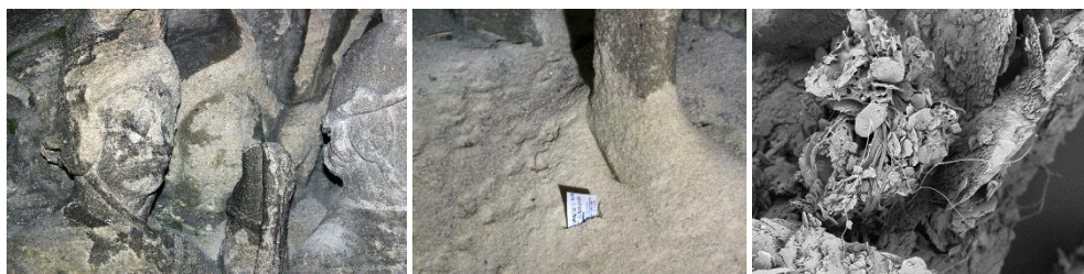
Fig.1: Details from previous state: Crusts and loss of material, decomposition and SEM image of a fragment with biogenic cover mixed with salt crystals.
