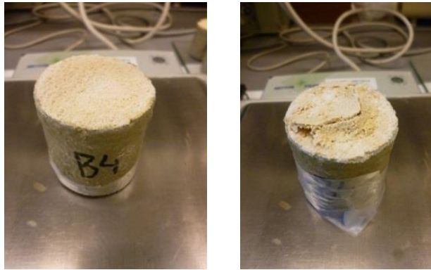
Fig. 14 Spalling of the reaggregated layer in a salt crystallisation test, after consolidation treatment (Bolhuis 2014)
