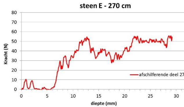
Fig. 7 DRMS profile of Lede sandy limestone, depth of degradation ca. 6 mm
