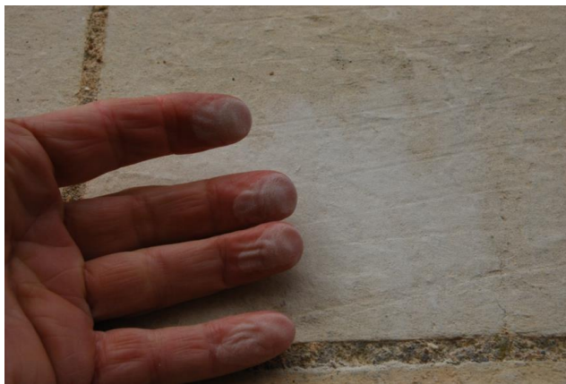
Fig. 1 Chalking of lime stone surface, photo from MDCS
