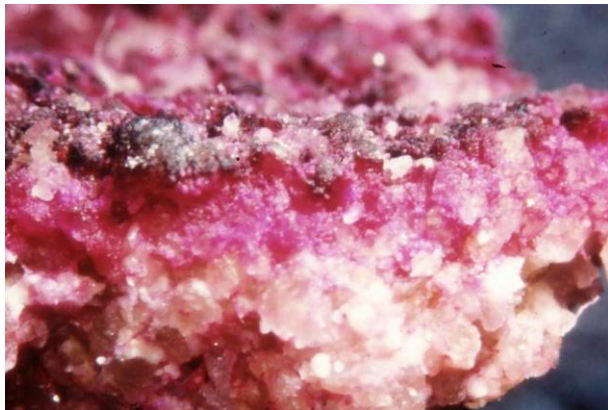
Fig. 1: Microbial biofilm penetrating into the pore system of a natural stone (e.g. Burgsandstein at Pommersfelden, Bavaria, Germany) as visualized by red PAS-staining.
