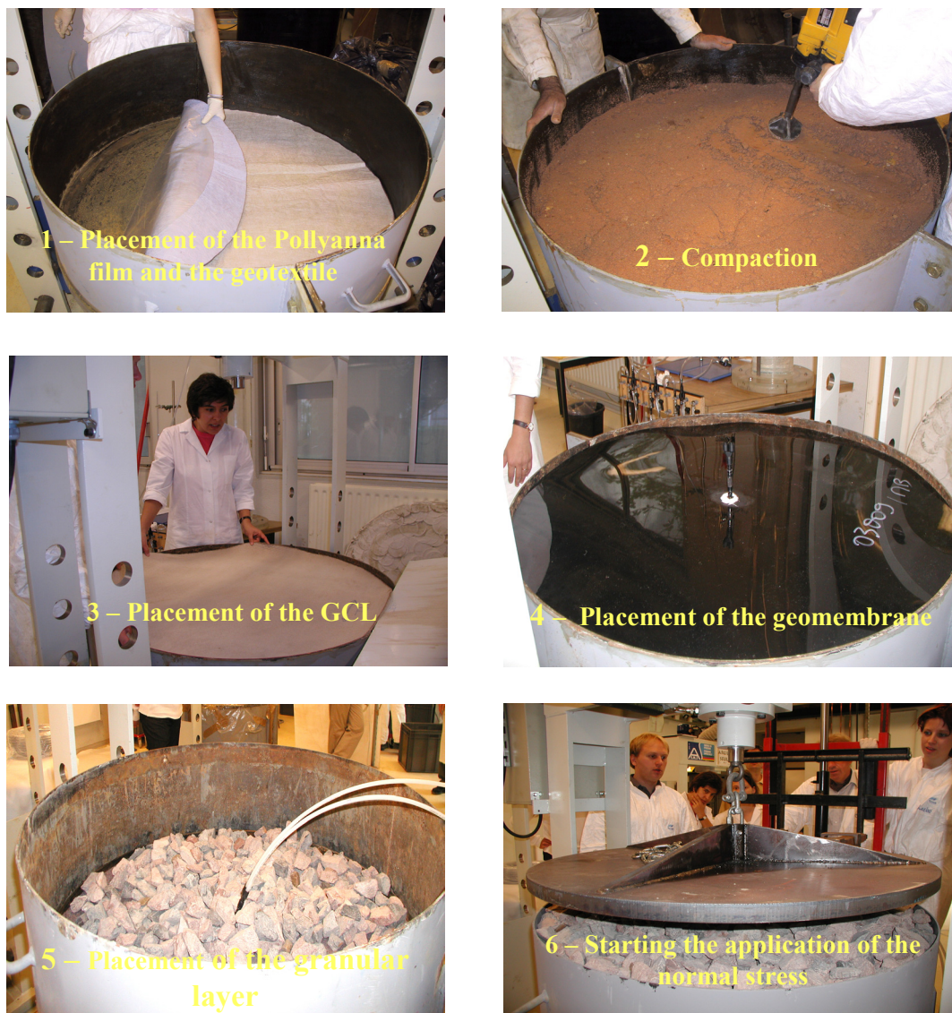
Figure 6.14 – Summary of intermediate-scale test procedure
