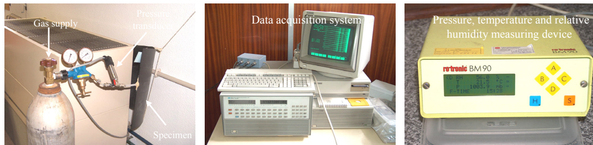
Figure 5.4 - Large-scale test assembly
