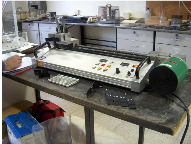
Figure 5.5 - Tensiometer used for performing the mechanical seam tests
