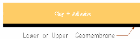
Figure 2.17 – Scheme of the geomembrane based GCLs (modified from Rollin et al. 2002a)
