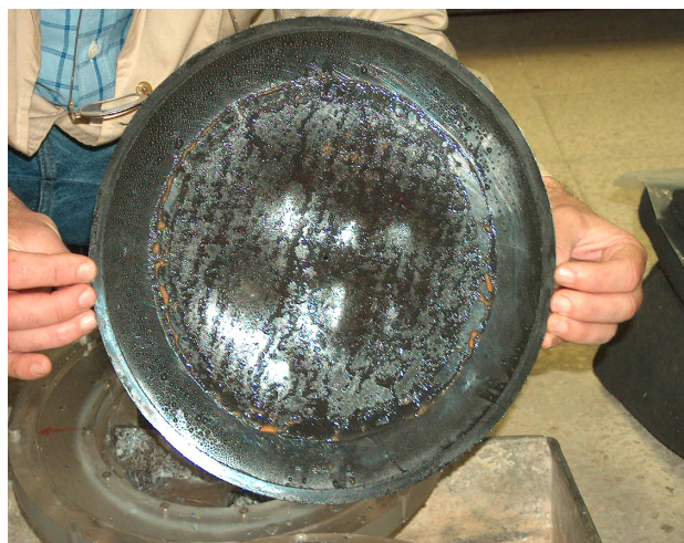
Figure 6.23 – Example of the geomembrane lower surface in contact with the GCL at the end of test 9
