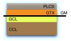
Figure 2: Landfill cut with a barrier system.
