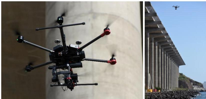
**Figure 7.** UAV system in flight to acquire aerial images.
