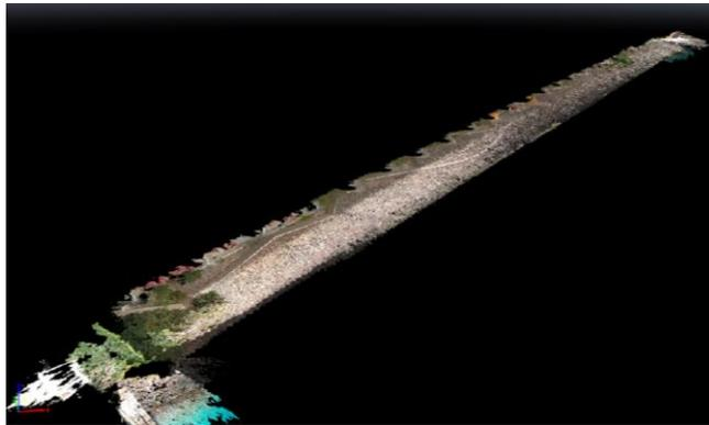
**Figure 10.** Resulting point clouds of the berm breakwater, April 2021.
