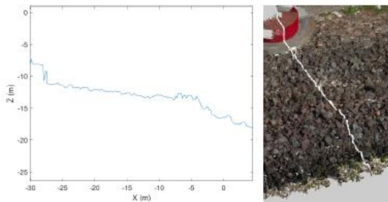
**Figure 13.** Example of berm breakwater profile and their approximate location (in white) in the point cloud.
