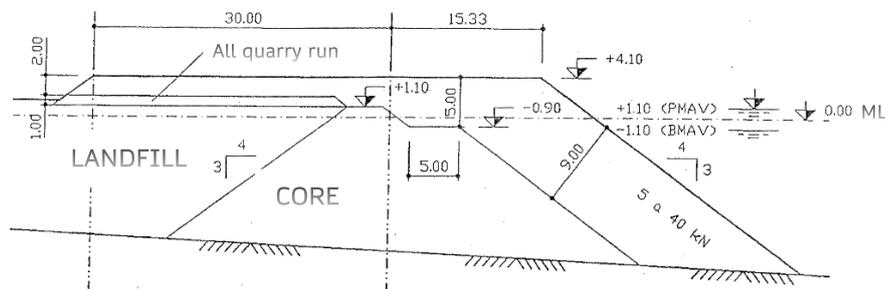
**Figure 2.** Cross-sectional profile of the berm breakwater (referred to ML).
