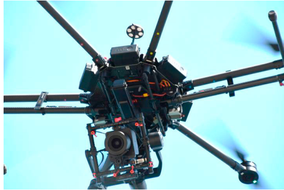
Fig. 1. The UAV system used in this project for image acquisition: DJI Matrice 600 Pro, with DJI Ronin MX gimbal and Phase One iXM-50 camera.
