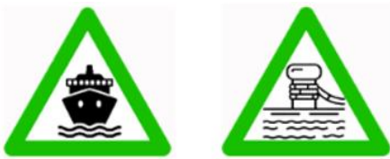
Figure 9. Symbols used by the SAFEPOR system to alert ships' motions danger (left) and ships' mooring systems failure danger (right).
