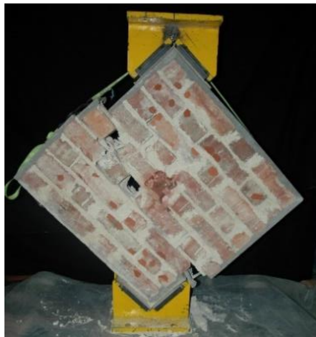
Figure 8. Collapse mode of the plain (non-strengthened) wallette M1M5.
