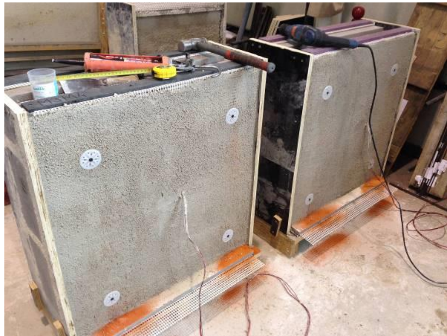
Figure 6. Wallettes with the reinforced render.
