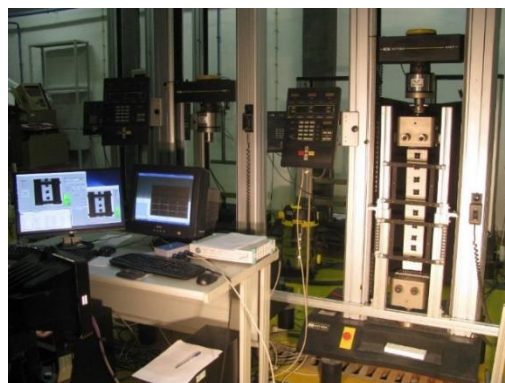
Figure 2. Execution of the tensile tests on reinforced mortar specimens.
