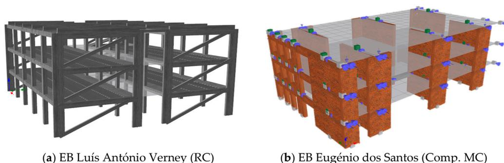
**Figure 6.** Nonlinear numerical models for structural response assessment at different levels of seismic action intensity for a: (a) RC structure; and (b) composite masonry–concrete structure.
