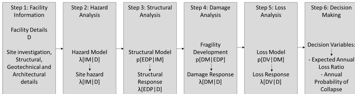
Figure 4. Illustration of the four stages of the PEER PBEE framework (adapted from [27]).
