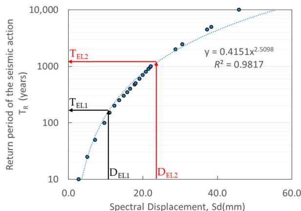
**Figure 8.** Structural response hazard curve—graphical representation of the procedure for calculating the return periods associated with the exceedance of the structural response limit states EL1 and EL2.
