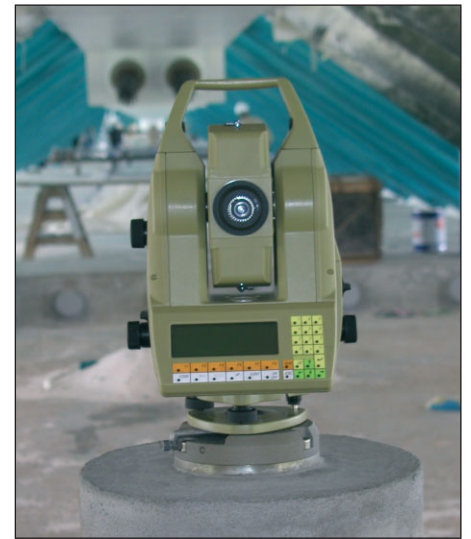
Fig. 7: Total station during load tests
