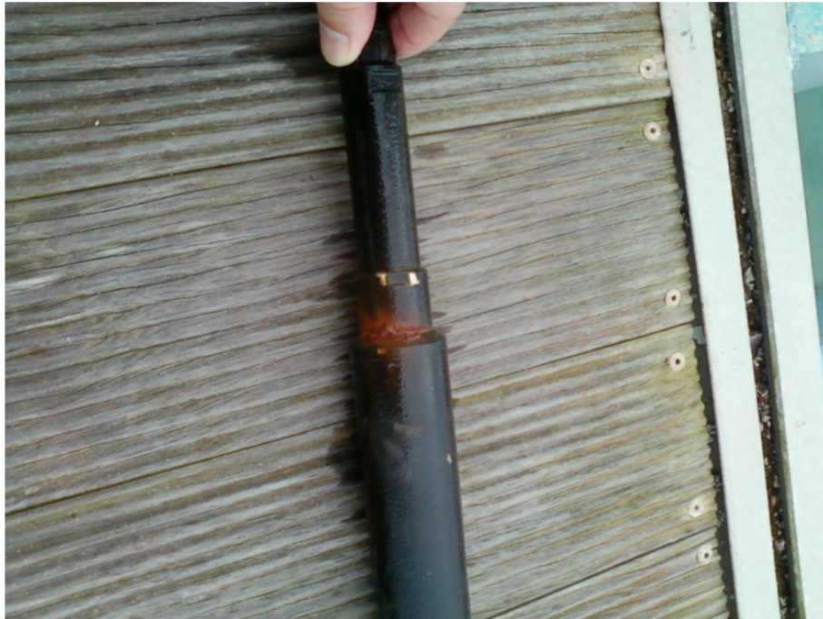
Figure 3.1: Oxidation of a water quality probe caused by the harsh aquatic environment.
