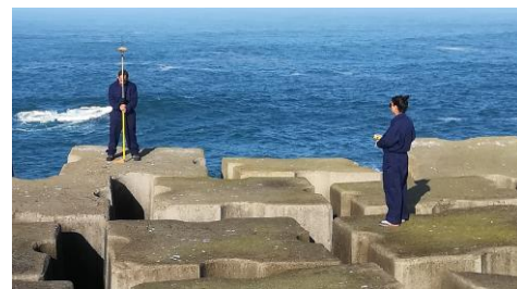
Figure 12 – Coordinating a GCP. The greenish colour of the surface of the blocks is due to slime
