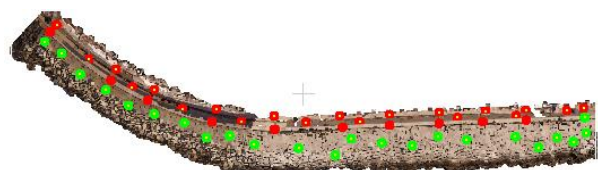
Figure 15 – Location of the GCP in breakwater C
